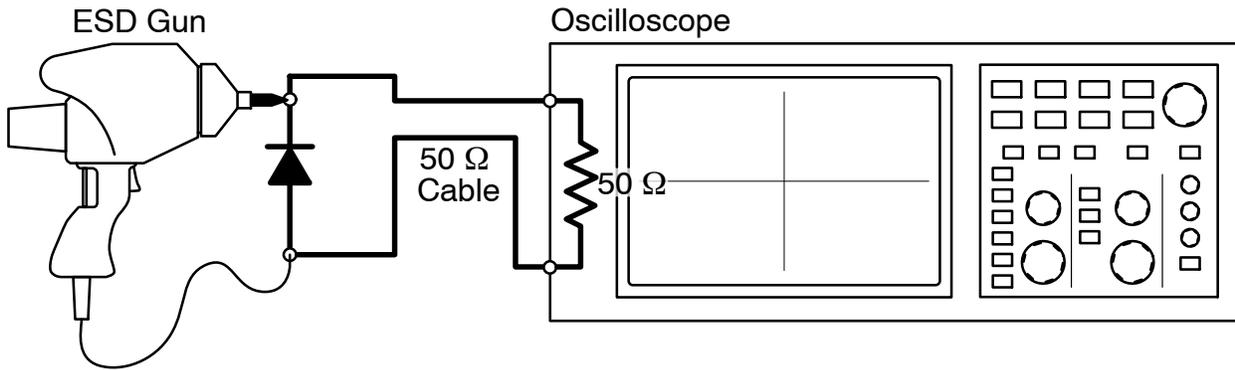
Figure 9. Diagram of ESD Clamping Voltage Test Setup
