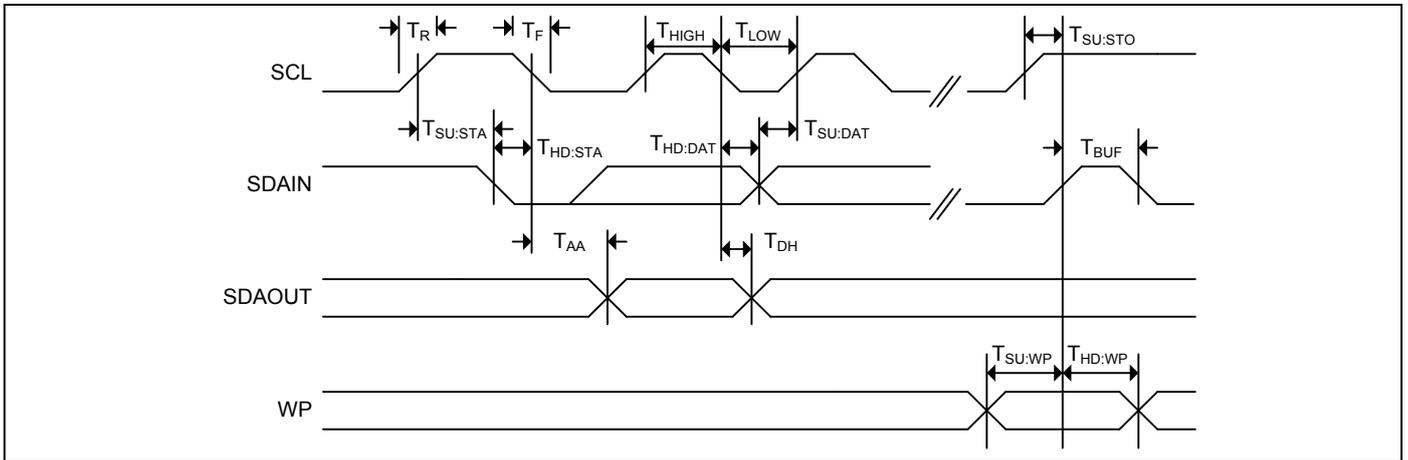
**Figure 5-12. Write Cycle Timing**
