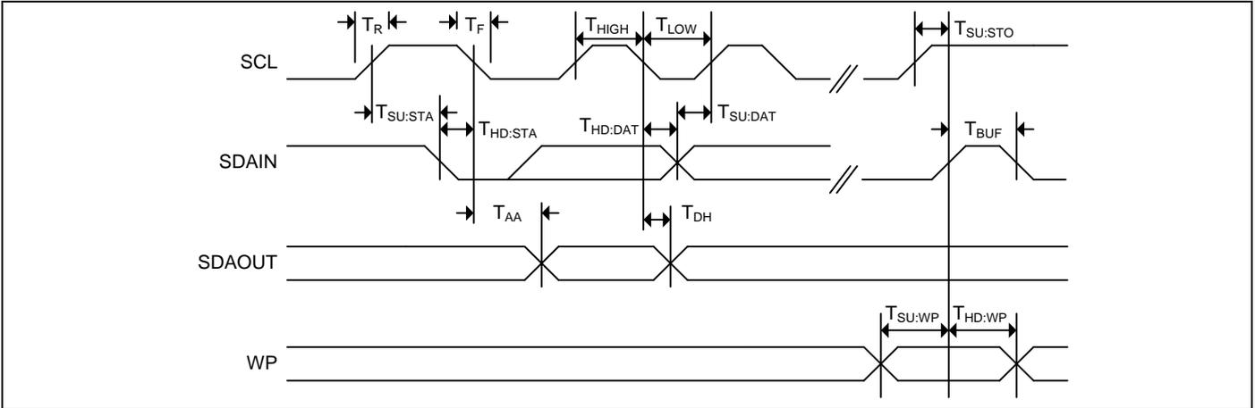
Figure 5-12. Write Cycle Timing
