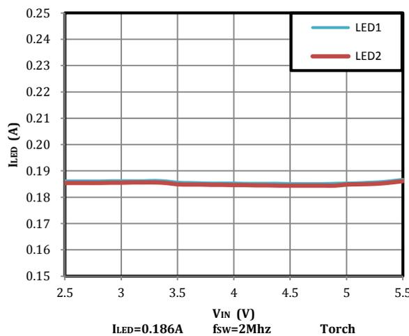
Fig 22. LED1 & LED2 Current vs Input Voltage
