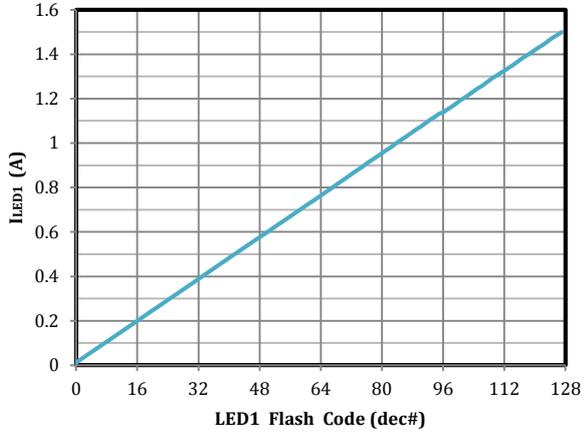
Fig 5. LED1 Flash Current vs Brightness Code
