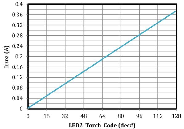
Fig 8. LED2 Torch Current vs Brightness Code
