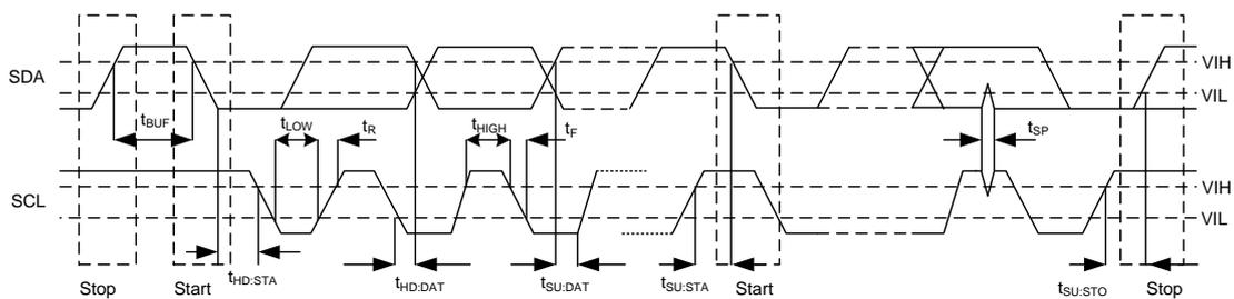
Fig 4 I<sup>2</sup>C INTERFACE TIMING
