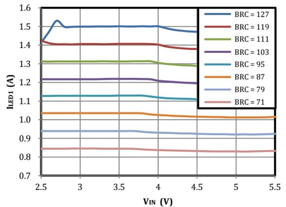
Fig 10. LED1 Flash Current vs Input Voltage
