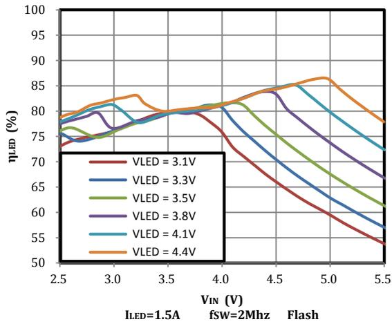
Fig23. LED Efficiency vs Input Voltage
