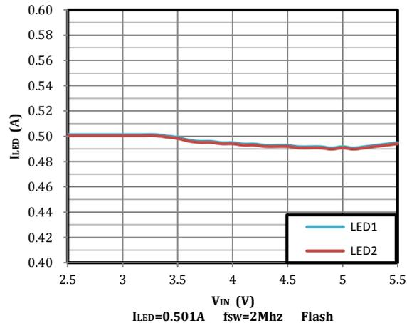
Fig 16. LED1 & LED2 Current vs Input Voltage
