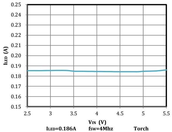
Fig 20. LED1/2 Torch Current vs Input Voltage
