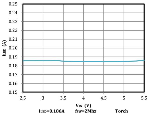
Fig 19. LED1/2 Torch Current vs Input Voltage
