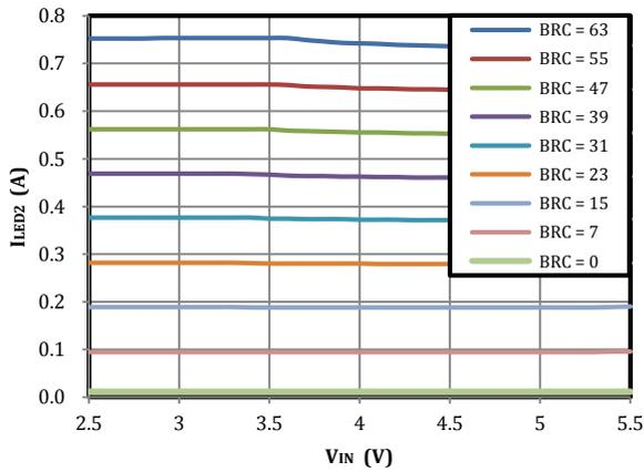
Fig 11. LED2 Flash Current vs Input Voltage
