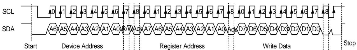
**Fig 55 I<sup>2</sup>C Write Timing**
