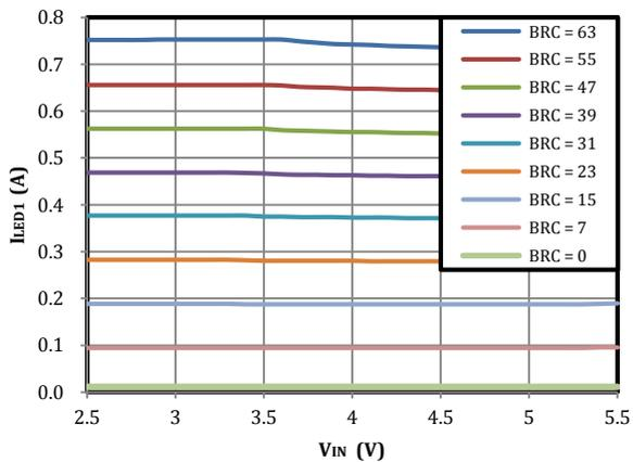
Fig 9. LED1 Flash Current vs Input Voltage
