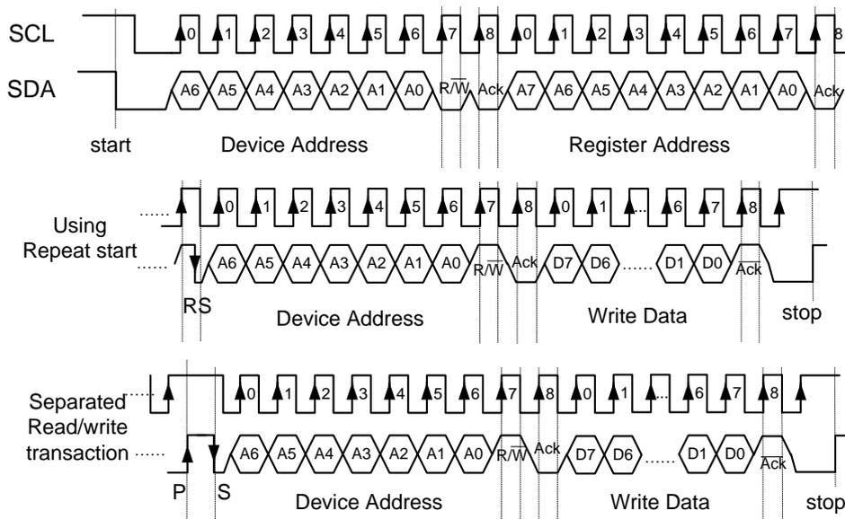
Fig 56 I<sup>2</sup>C Read Timing
