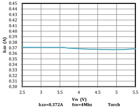
Fig 18. LED1/2 Torch Current vs Input Voltage
