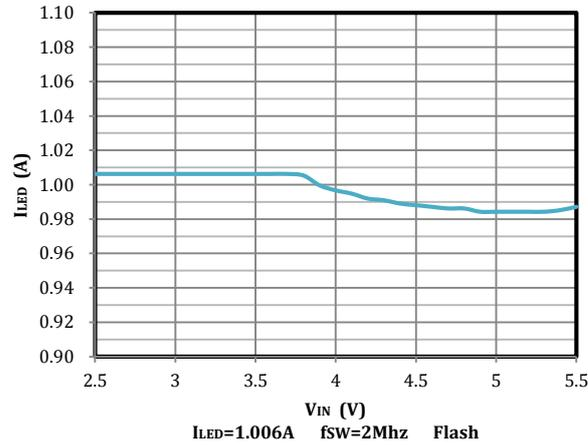
Fig 14. LED1/2 Flash Current vs Input Voltage
