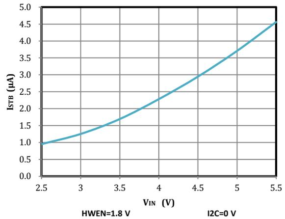
Fig 32. Standby Current vs Input Voltage
