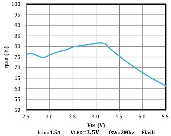
Fig24. LED Efficiency vs Input Voltage
