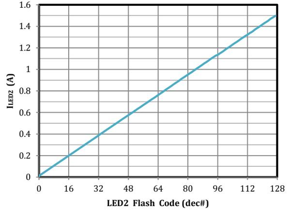
Fig 6. LED2 Flash Current vs Brightness Code
