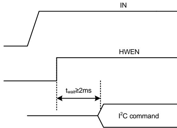
**Fig 46 Power-Up Sequence with HWEN Driven by GPIO**
