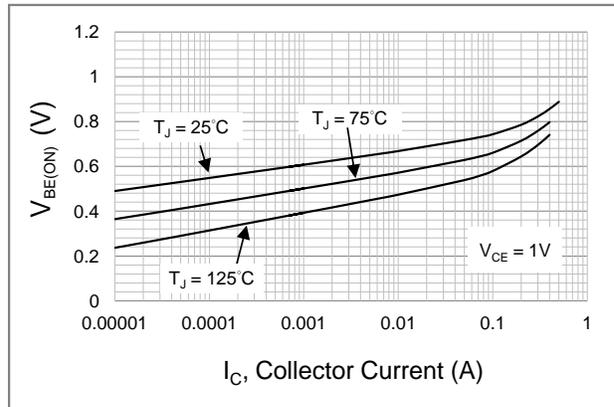
Fig.4 Typical Base - Emitter Voltage vs Collector Current
