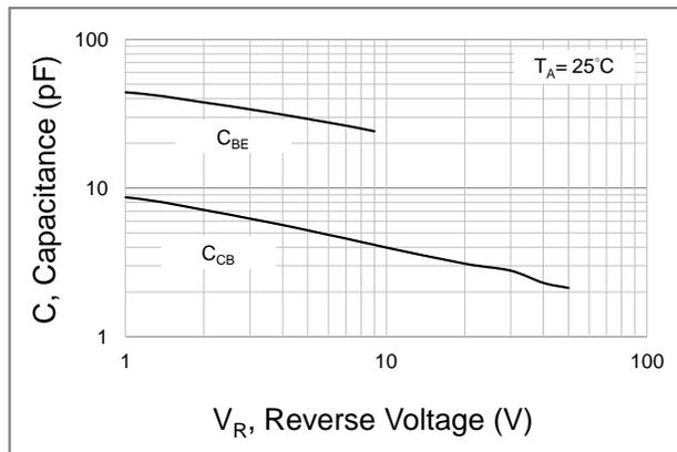
Fig.5 Typical Capacitance
