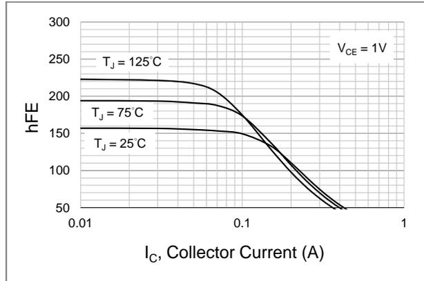
Fig.2 Typical DC Current Gain vs Collector Current
