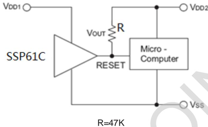
NMOS open drain output application with R-C delay
