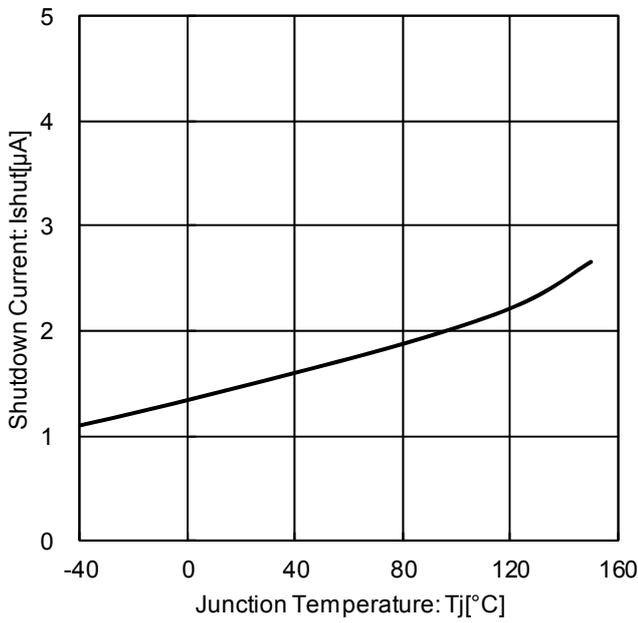
Figure 39. Shut Down Current vs. Temperature (CTL = 0 V)
