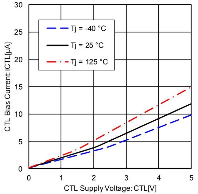
Figure 40. CTL Bias Current vs. CTL Supply Voltage
