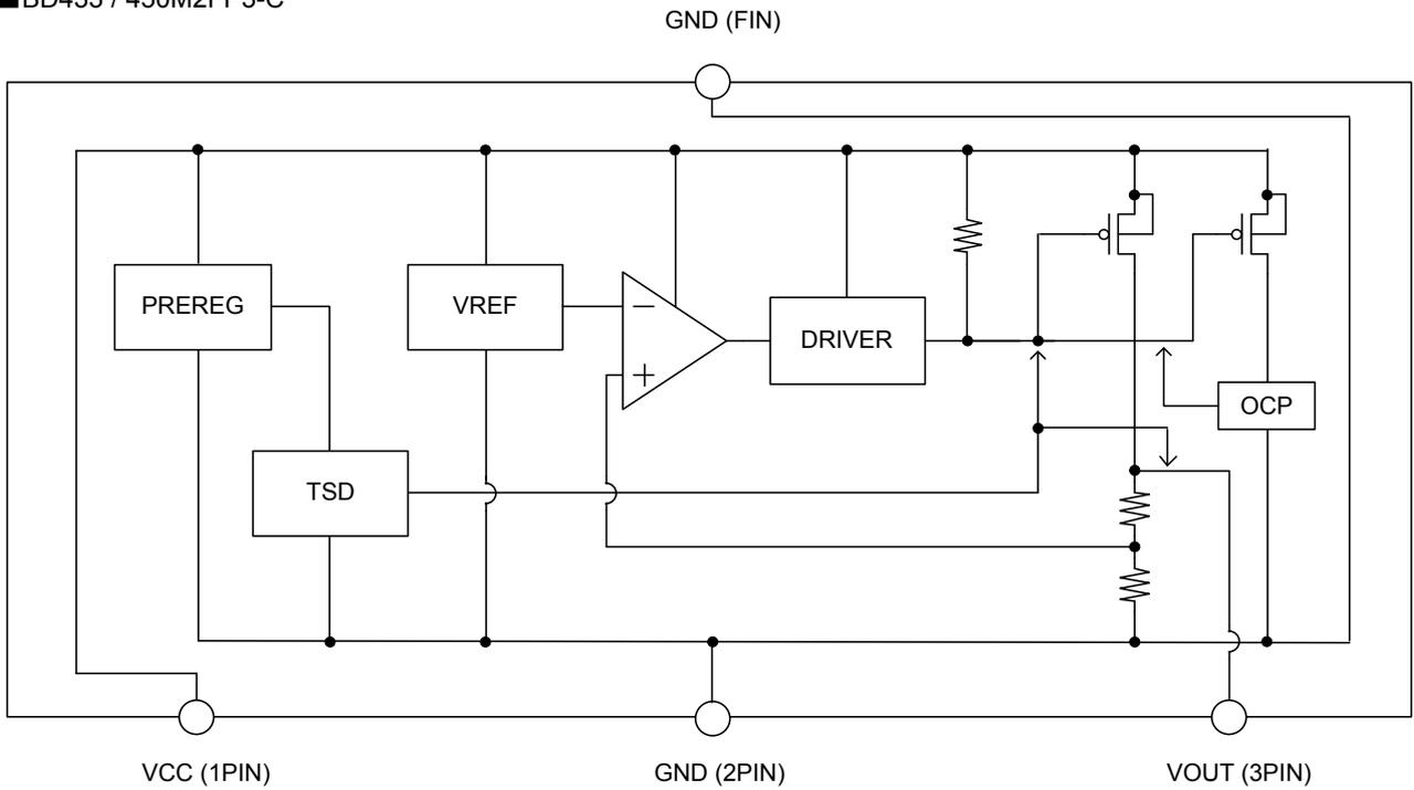
Figure 4. Block Diagrams
