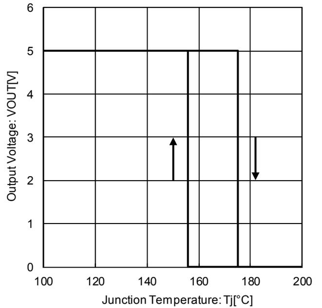
Figure 32. Output Voltage vs. Temperature (Thermal Shut Down)
