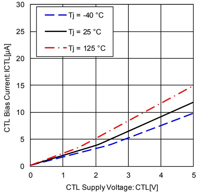
Figure 22. CTL Bias Current vs. CTL Supply Voltage
