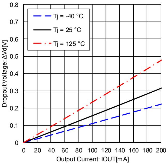
Figure 29. Dropout Voltage ( $V_{CC} = 4.75\text{ V}$ )
