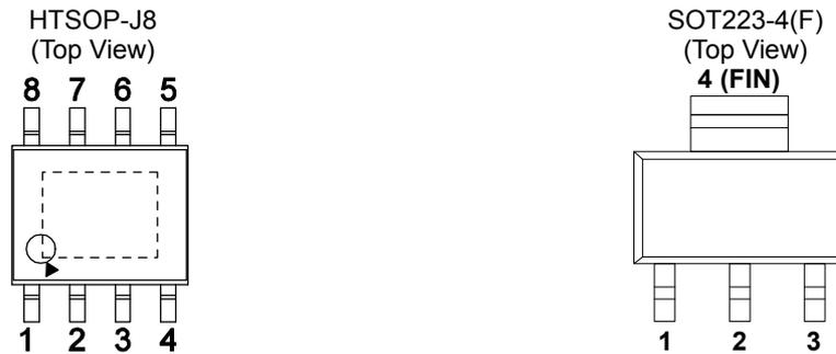
Figure 3. Pin Configuration
