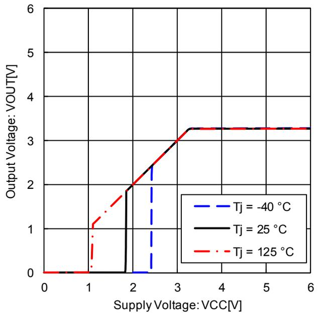
Figure 8. Output Voltage vs. Power Supply Voltage (IOUT = 0 mA)
