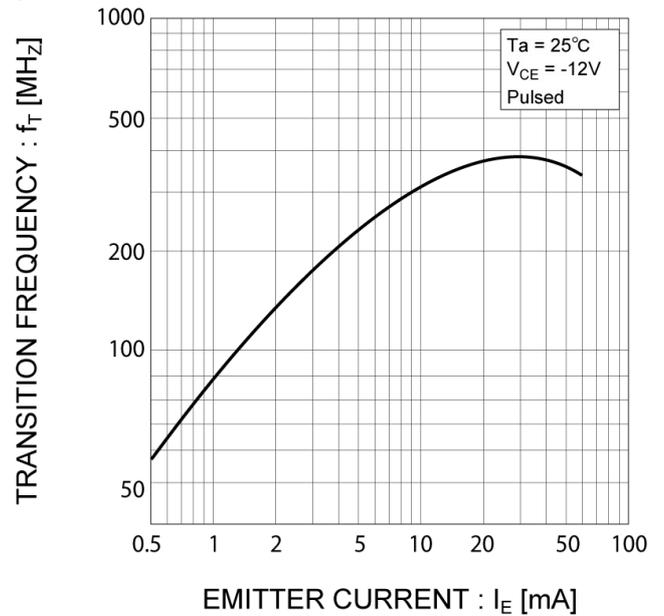
●Electrical characteristic curves( $T_a = 25^\circ\text{C}$ )
