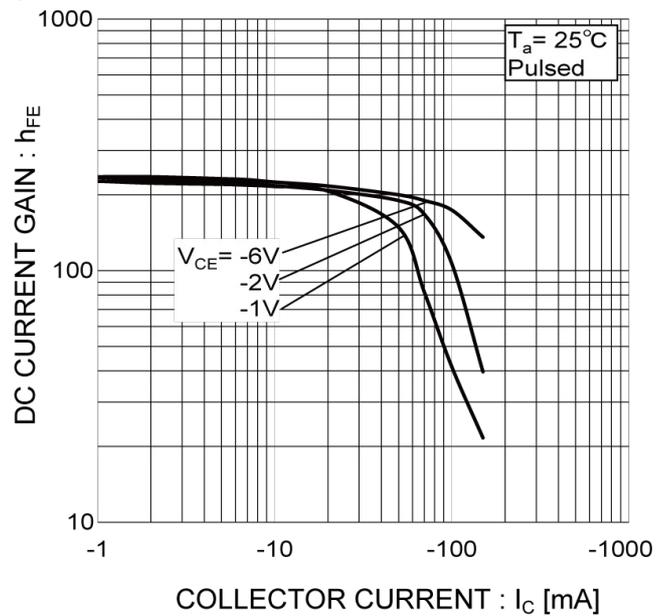
●Electrical characteristic curves( $T_a = 25^\circ\text{C}$ )
