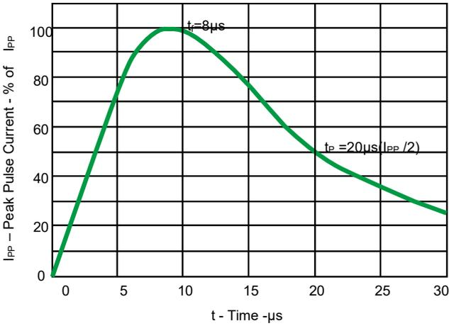
Fig 1. Pulse Waveform
