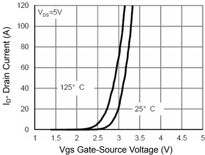
Figure 2 Transfer Characteristics
