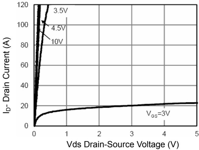
Figure 1 Output Characteristics
