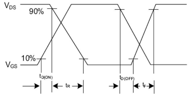
Fig. 2.2 Switching Waveforms
