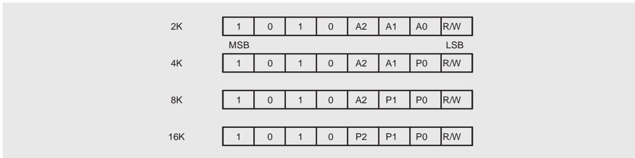
Figure 5: Byte Write
