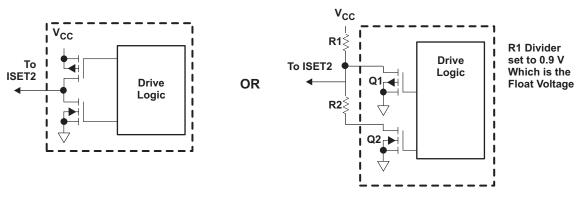
Figure 12. 3-State ISET2 Terminal Circuits
