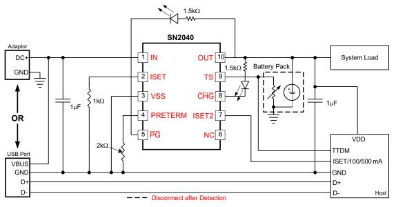
Figure 14. Typical Application Circuit
