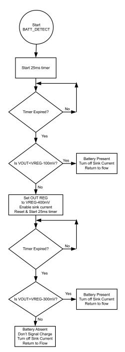
Figure 13. Battery Detect Routine
