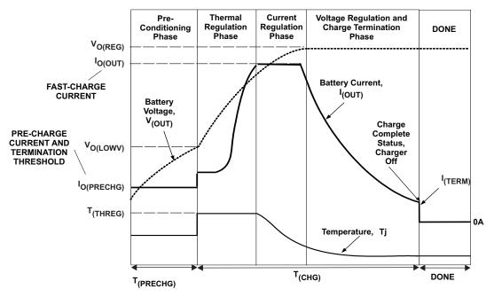
Figure 7. Charging Profile With Thermal Regulation
