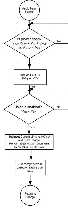
Figure 9. SN2040 Power-Up Flow Diagram
