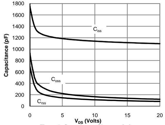
Figure 8: Capacitance Characteristics
