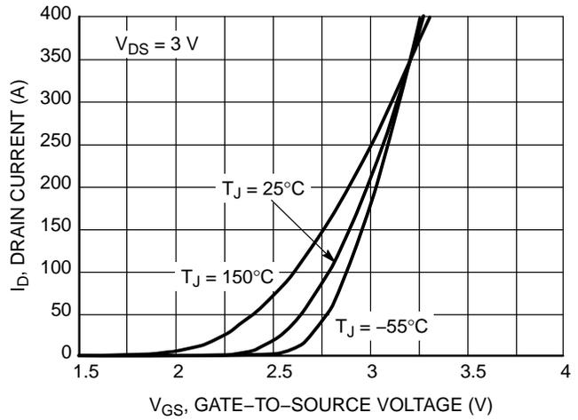
Figure 2. Transfer Characteristics
