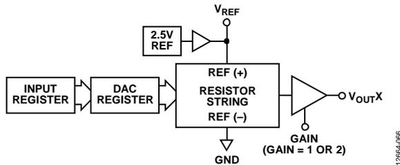
Figure 55. Single DAC Channel Architecture Block Diagram
