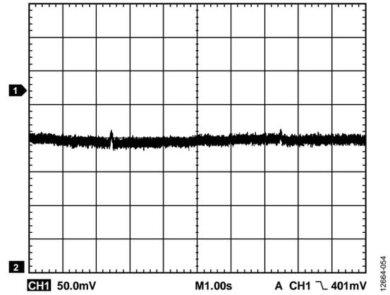
Figure 45. 0.1 Hz to 10 Hz Output Noise Plot
