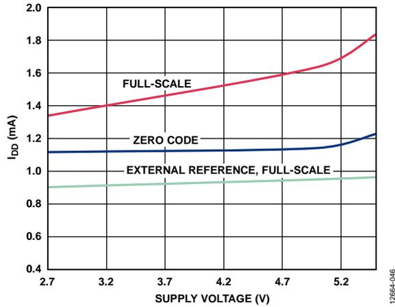
Figure 37.  $I_{DD}$  vs. Supply Voltage
