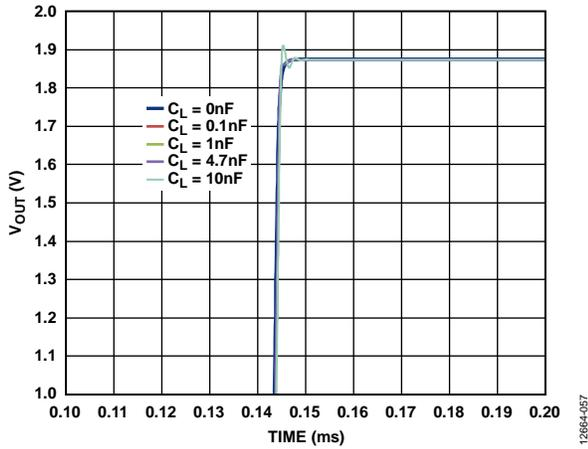
Figure 48. Settling Time at Various Capacitive Loads
