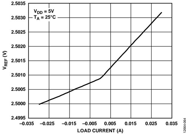
Figure 53.  $V_{REF}$  vs. Load Current and  $V_{DD}$
