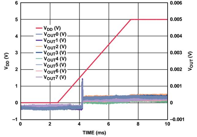
Figure 40. Power-On Reset to 0 V and Midscale
