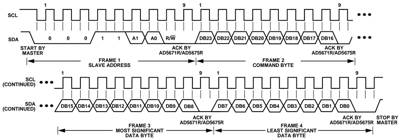
Figure 59. I<sup>2</sup>C Write Operation
