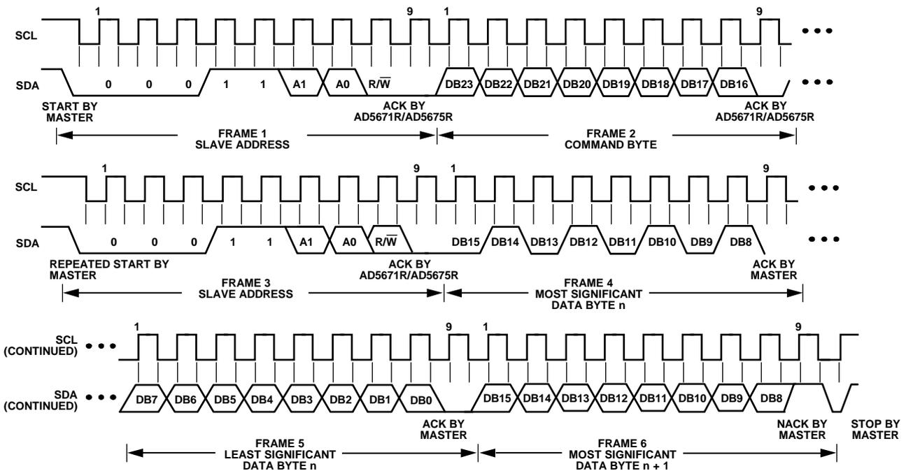
Figure 60. I<sup>2</sup>C Read Operation
