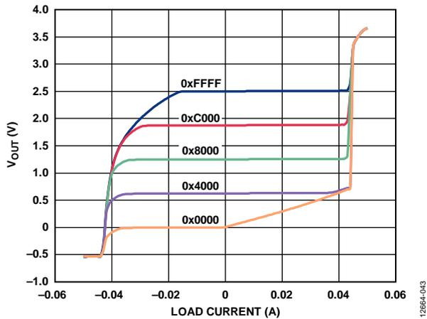
Figure 34. Source and Sink Capability at 3 V
