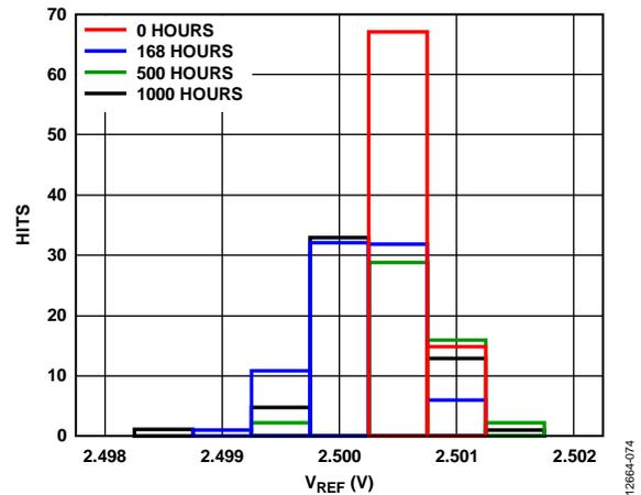
Figure 64. Reference Drift Through to 1000 Hours
