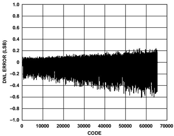
Figure 8. AD5675R DNL Error vs. Code
