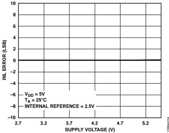
Figure 13. AD5671R INL Error vs. Supply Voltage
