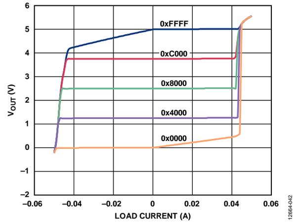
Figure 33. Source and Sink Capability at 5 V
