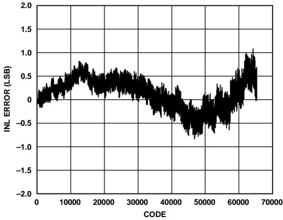
Figure 6. AD5675R INL Error vs. Code
