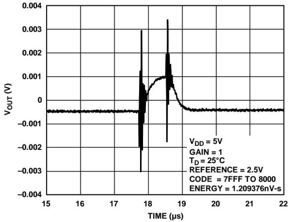
Figure 42. Digital-to-Analog Glitch Impulse
