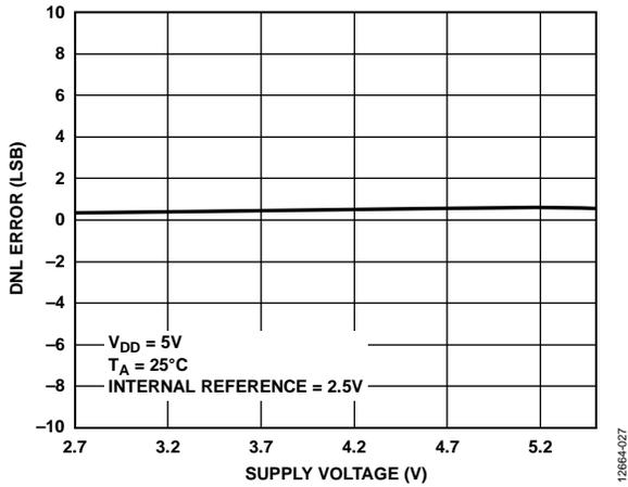
Figure 19. AD5675R DNL Error vs. Supply Voltage
