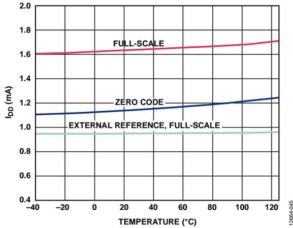
Figure 36.  $I_{DD}$  vs. Temperature
