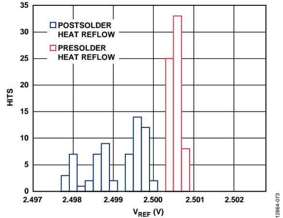
Figure 63. Solder Heat Reflow Reference Voltage Shift
