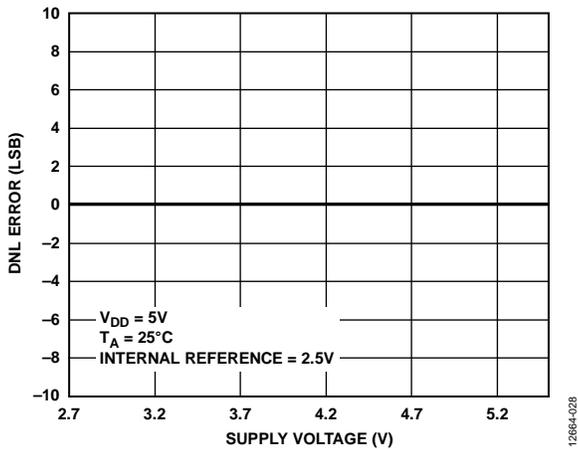
Figure 20. AD5671R DNL Error vs. Supply Voltage
