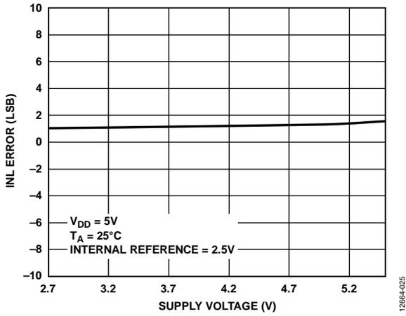
Figure 18. AD5675R INL Error vs. Supply Voltage
