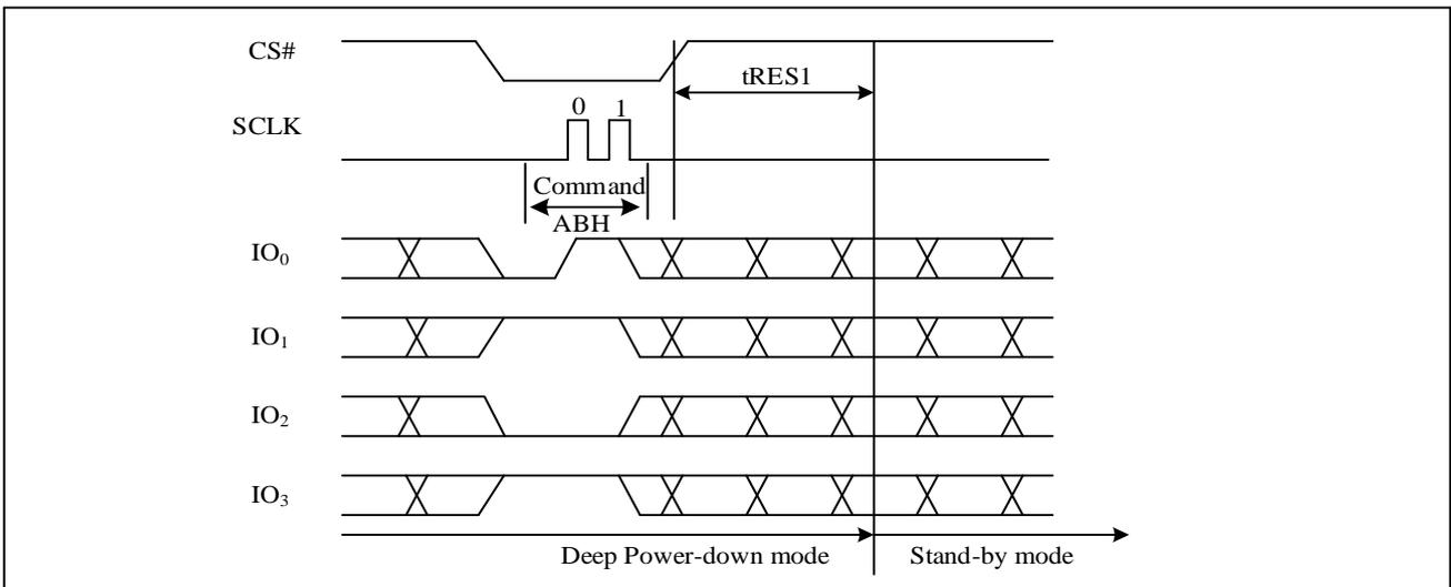
Figure23. Release Power-Down/Read Device ID Sequence Diagram
