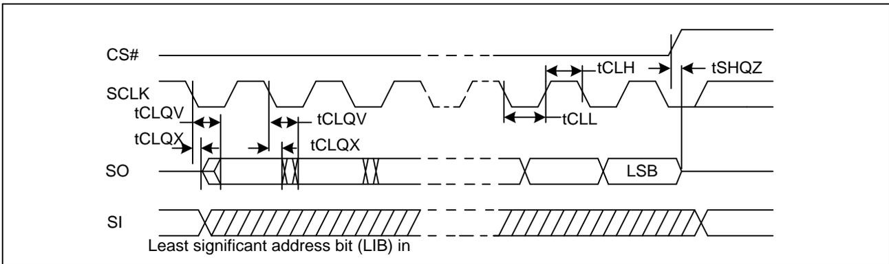
Figure45. Resume to Suspend Timing
