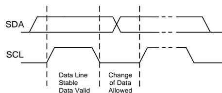
Fig 52 Data Validation Diagram
