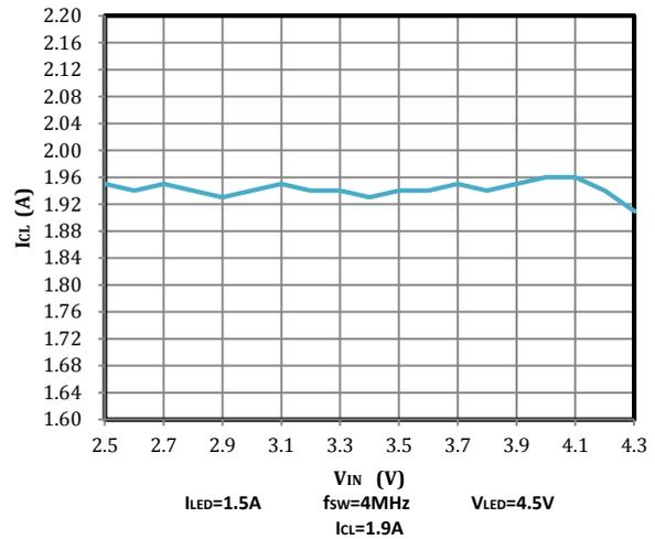
Fig 36. Inductor Current Limit vs Input Voltage
