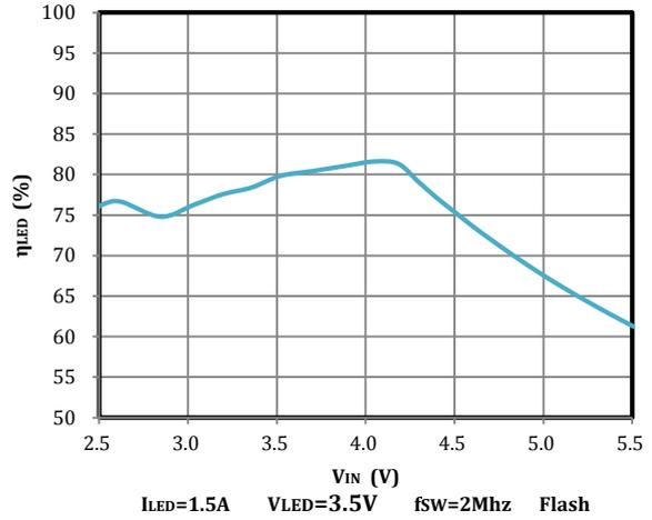
Fig24. LED Efficiency vs Input Voltage
