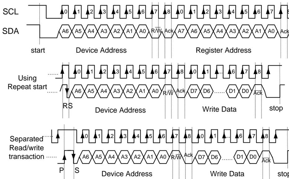
Fig 56 I<sup>2</sup>C Read Timing
