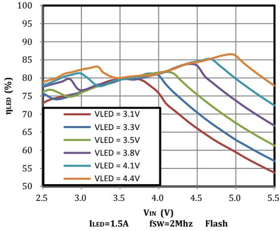
Fig23. LED Efficiency vs Input Voltage
