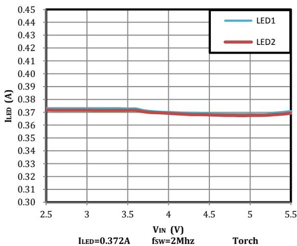
Fig 21. LED1 & LED2 Current vs Input Voltage
