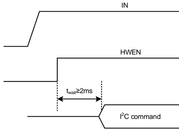
**Fig 46 Power-Up Sequence with HWEN Driven by GPIO**
