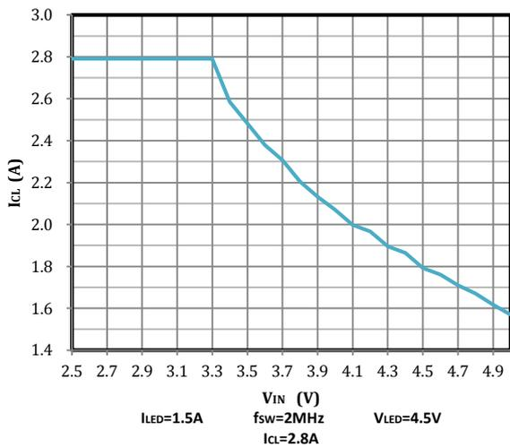
Fig 37. Inductor Current Limit vs Input Voltage
