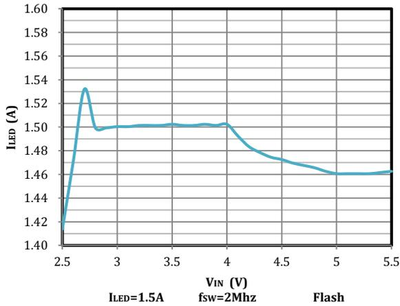
Fig 13. LED1/2 Flash Current vs Input Voltage
