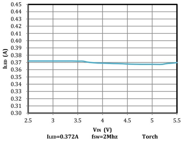
Fig 17. LED1/2 Torch Current vs Input Voltage
