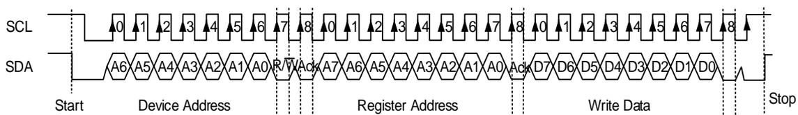
**Fig 55 I<sup>2</sup>C Write Timing**
