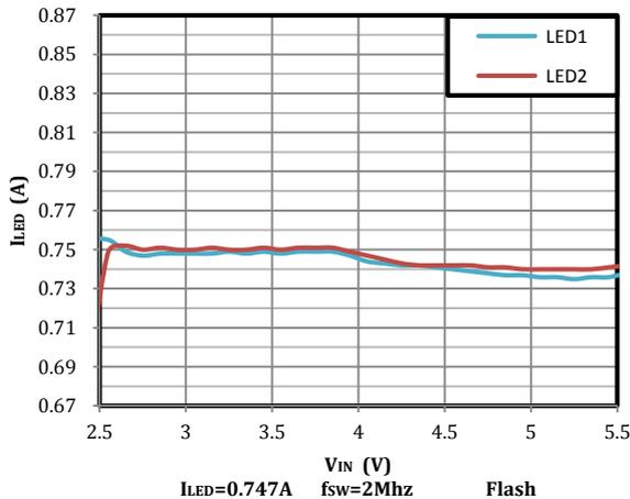
Fig 15. LED1 & LED2 Current vs Input Voltage
