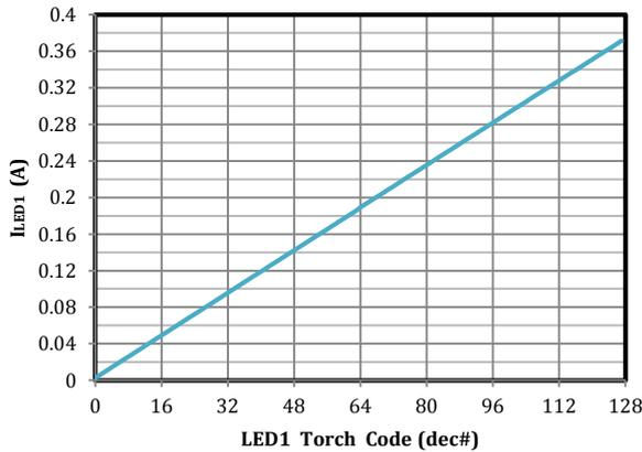
Fig 7. LED1 Torch Current vs Brightness Code
