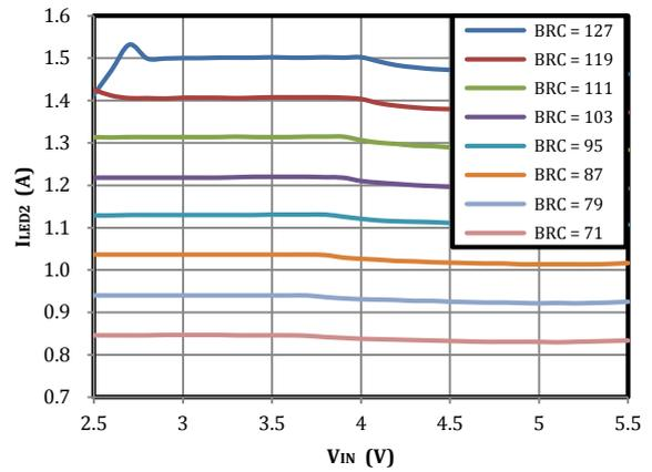
Fig 12. LED2 Flash Current vs Input Voltage
