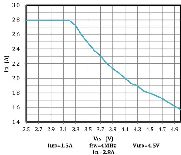
Fig 38. Inductor Current Limit vs Input Voltage
