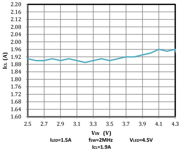
Fig 35. Inductor Current Limit vs Input Voltage
