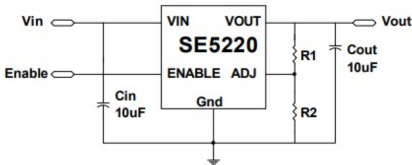
$$V_{out} = 0.8 * (1 + R1/R2) \text{ Volts}$$
