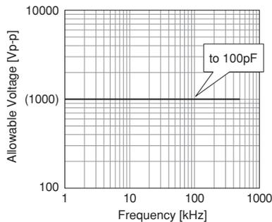
The sine-wave frequency VS allowable voltage
