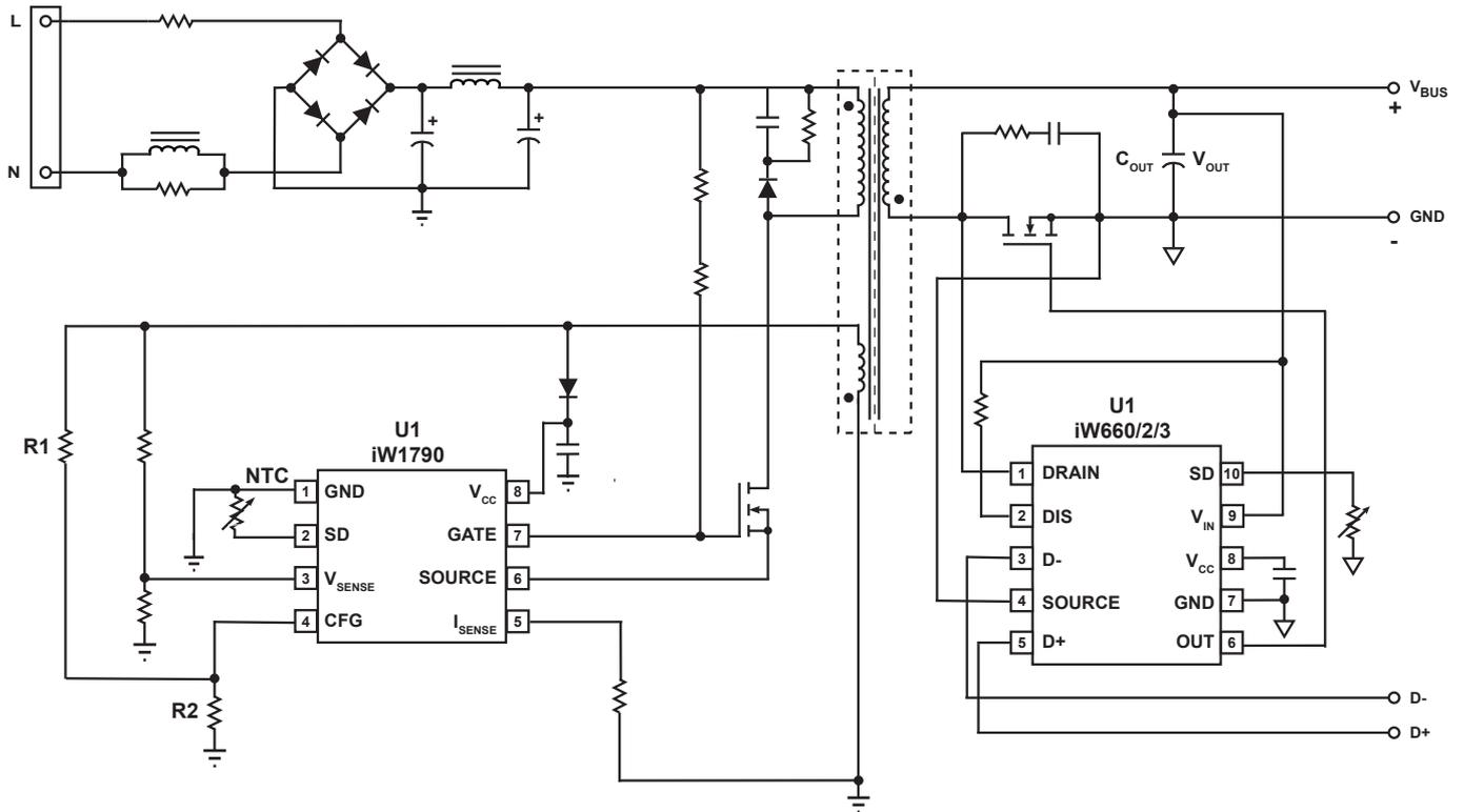
**Figure 2.1 : iW1790 Typical Application Circuit for Multi-Level Output Voltage and Current (Using iW660/2/3 as Secondary-Side Controller for Rapid Charge Protocols. Achieving < 20mW No-Load Power Consumption in Typical 15W Design.)**
