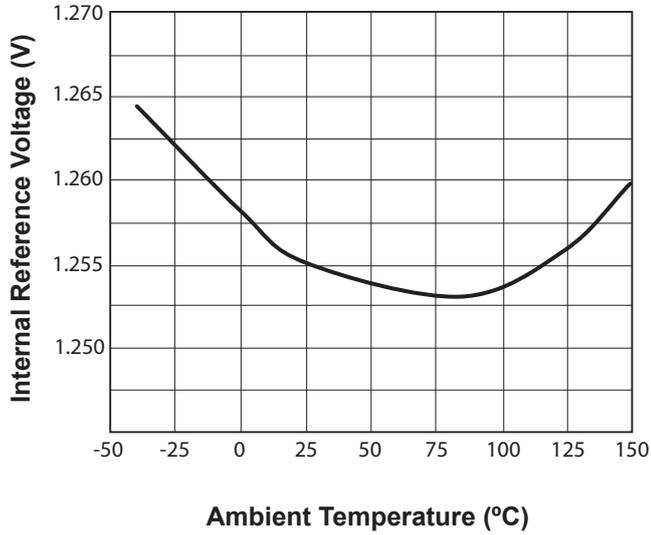
Figure 7.1 : Internal Reference Voltage vs. Ambient Temperature
