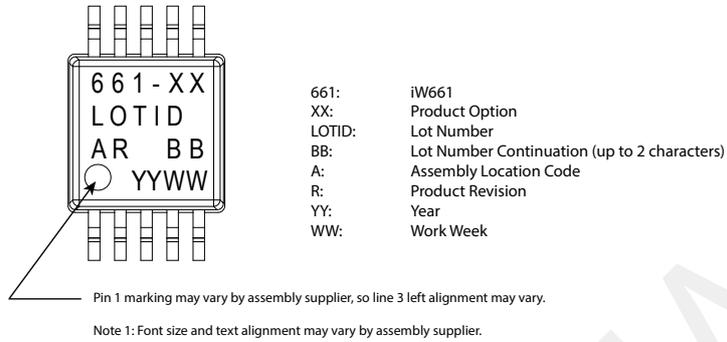
**Figure 12.1 : Top Marking for the iW661**
