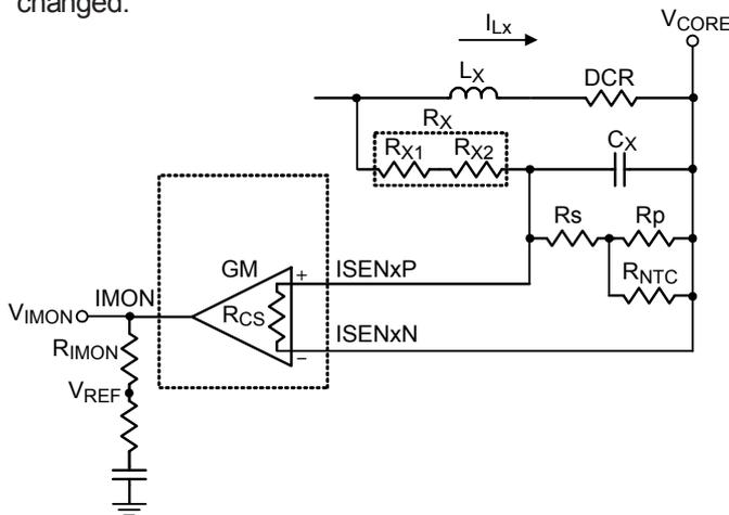
Figure 13. Thermal Compensation method for Single Phase
