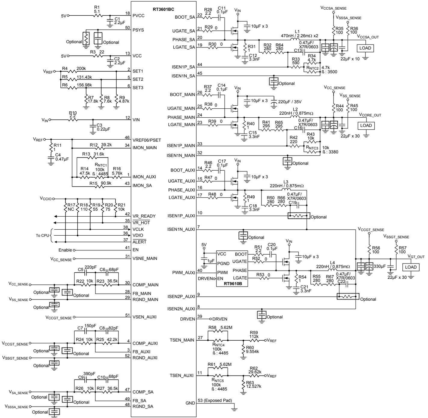
Note : R22 to R27, C5 to C10 customer must to tune final parameters on system board at first time.
