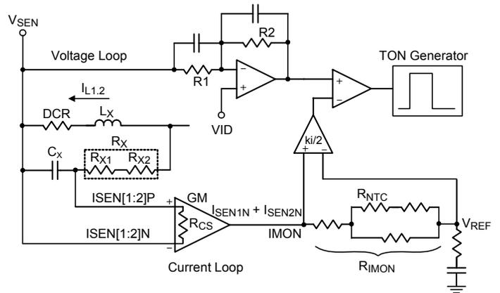
Figure 17. Voltage Loop and Current Loop for AUXI
