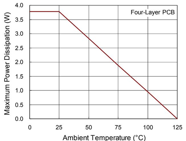
Figure 27. Derating Curve of Maximum Power Dissipation
