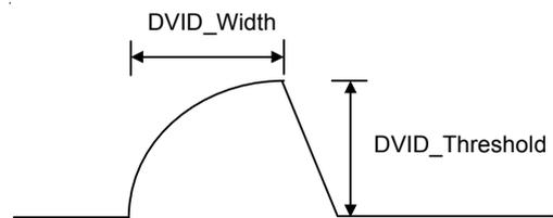
Figure 22. Definition of Virtual Charge Current Signal
