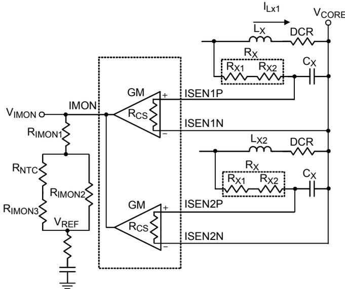
Figure 14. Thermal Compensation method for dual Phase
