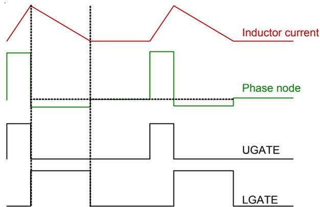
Figure 2. Diode Emulation Mode (DEM) in Steady State
