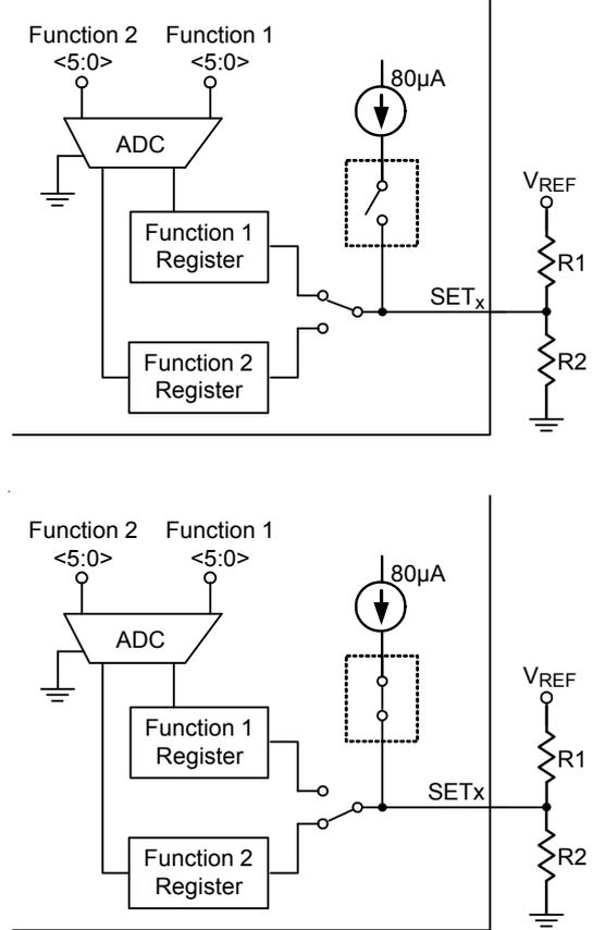
Figure 4. Multi-Function Pin Setting Mechanism for SET [1:3]
