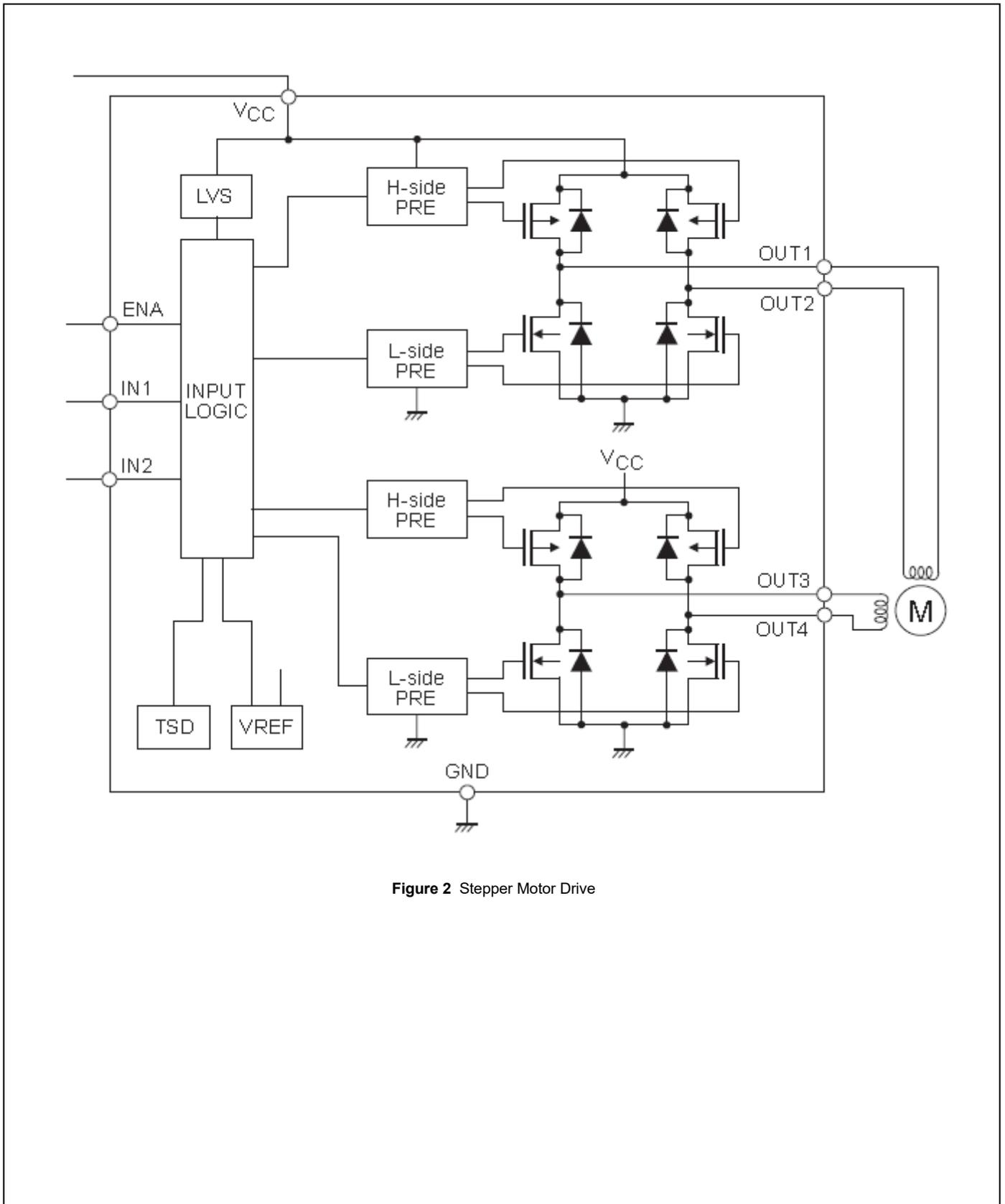
Figure 2 Stepper Motor Drive
