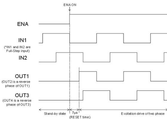
Figure 4 Control Timing
