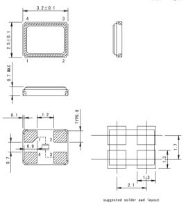
Note) #2, #4 is connected with a cover (Please connect with a GND or a power supply)
