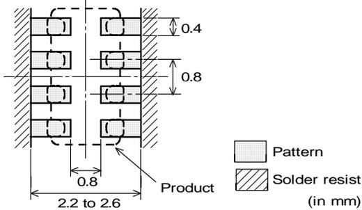
\* The excessive heat by land pads may cause deterioration at joint of products with substrate.
