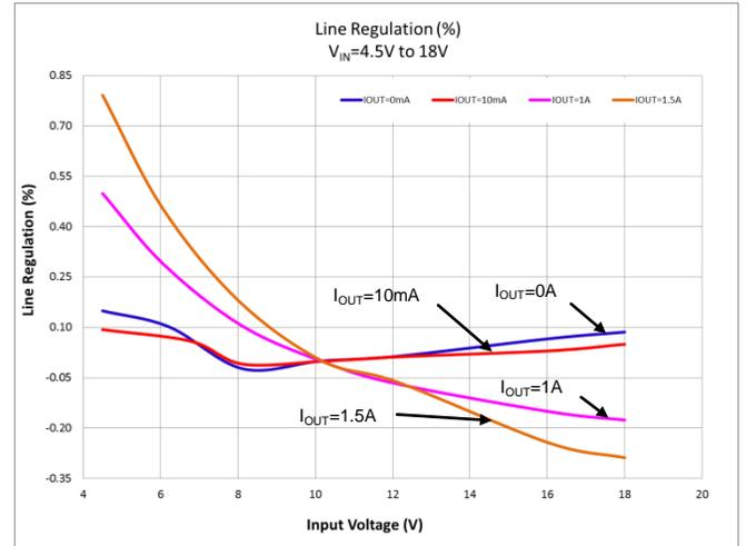
**Typical Performance Characteristics** (Cont.) (@ $T_A = +25^\circ\text{C}$ ,  $V_{IN} = 12\text{V}$ ,  $V_{OUT} = 3.3\text{V}$ ,  $L = 6.5\mu\text{H}$ ,  $C_1 = 22\mu\text{F}$ ,  $C_2 = 22\mu\text{F}$ , unless otherwise specified.)
