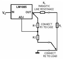
The LM1085 series develops a 1.25V reference voltage between the output and the adjust terminal. Placing a resistor between these two terminals causes a constant current to flow through R1 and down through R2 to set the overall output voltage.
