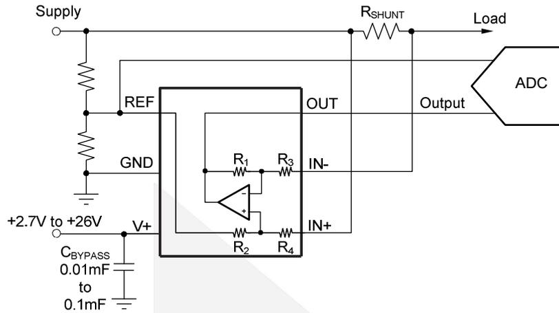
**Figure 13. Sensing DIO2388x to Cancel Effects of Impedance on the REF Input**
