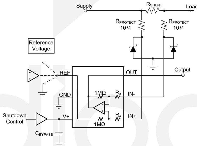
**Figure 14. DIO2388x Transient Protection Using Dual Zener Diodes**
