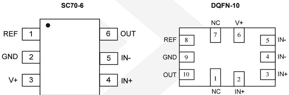
Figure 1 Pin Assignment
