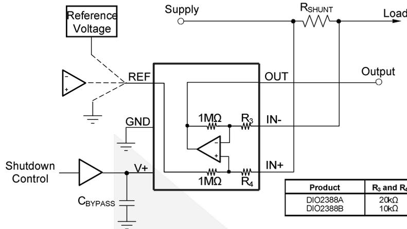
**Figure 12. Basic Circuit for Shutting Down DIO2388x with Grounded Reference**
