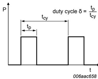
Fig. 13. Duty cycle definition
