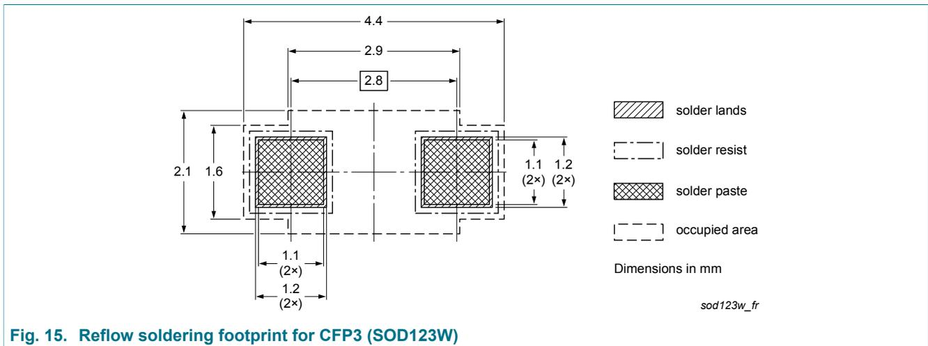
Fig. 15. Reflow soldering footprint for CFP3 (SOD123W)
