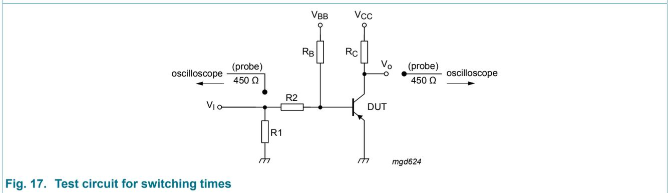
Fig. 17. Test circuit for switching times
