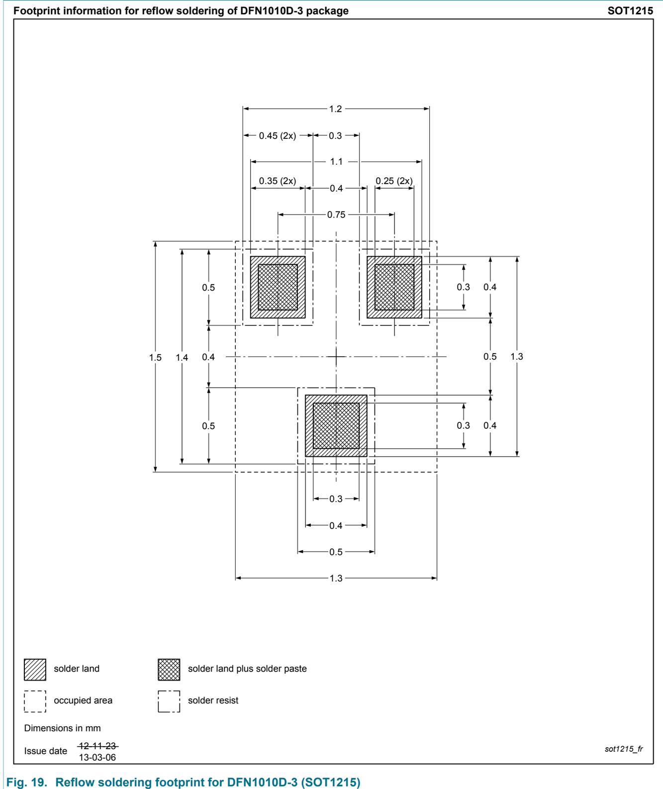
Fig. 19. Reflow soldering footprint for DFN1010D-3 (SOT1215)
