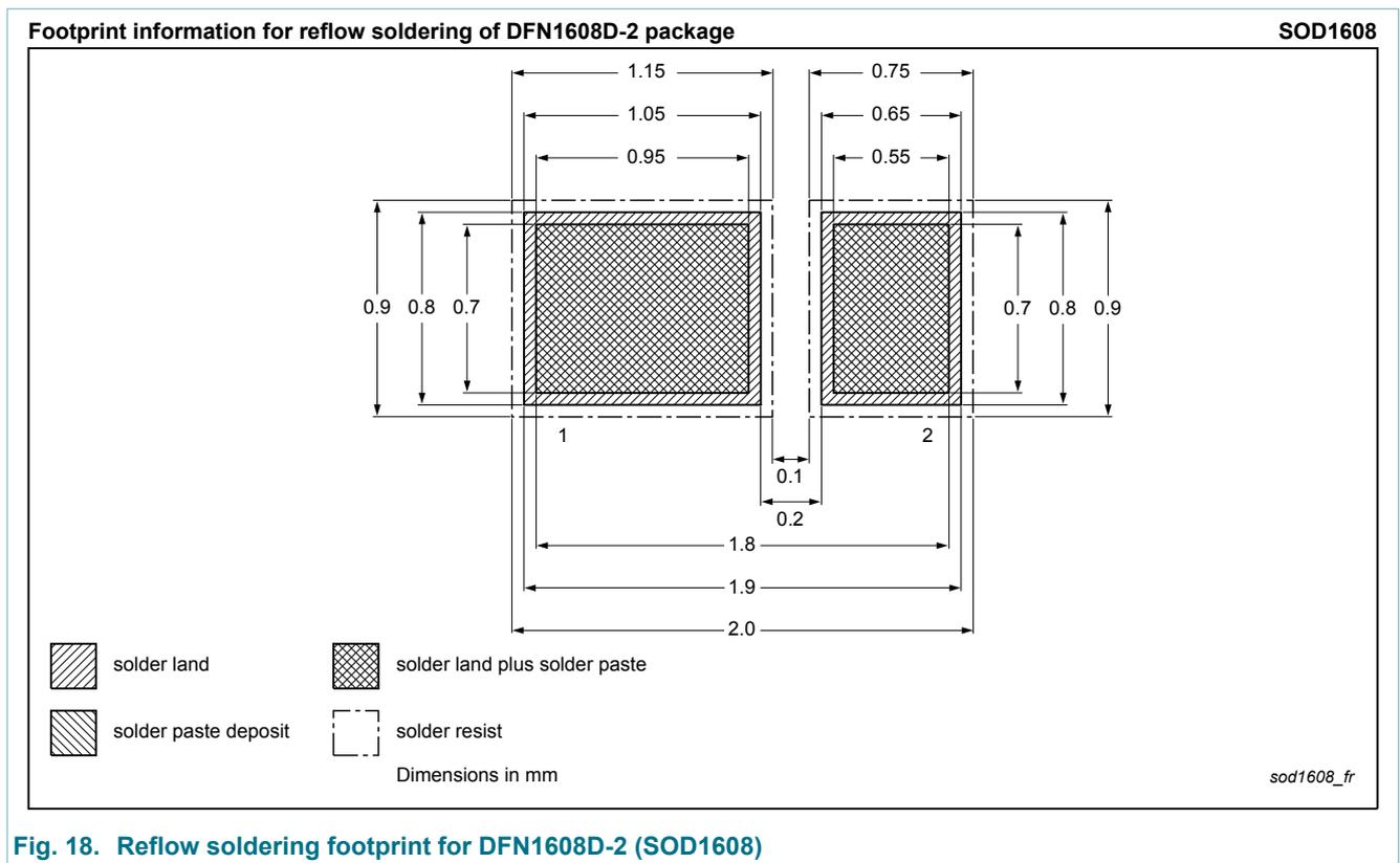
Fig. 18. Reflow soldering footprint for DFN1608D-2 (SOD1608)
