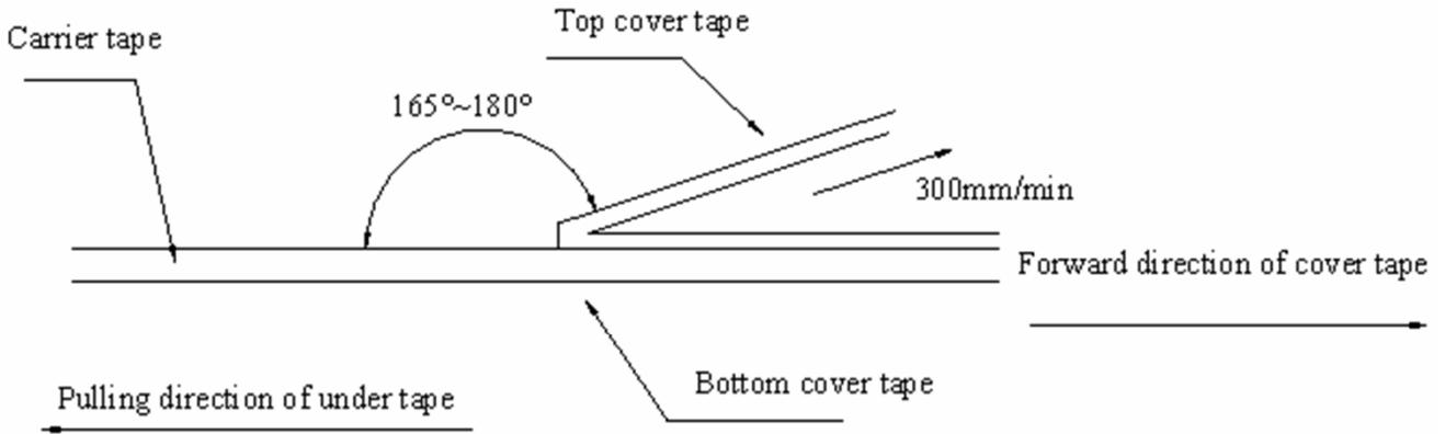
\*\*\* In the case, the cover tape is pulled off under the above conditions, the cover tape adhesion strength should be 10.2g~71.4g Plastic tape:10.2g~71.4g
