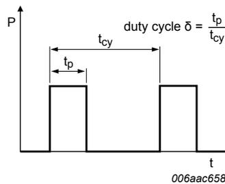
Fig. 16. Duty cycle definition
