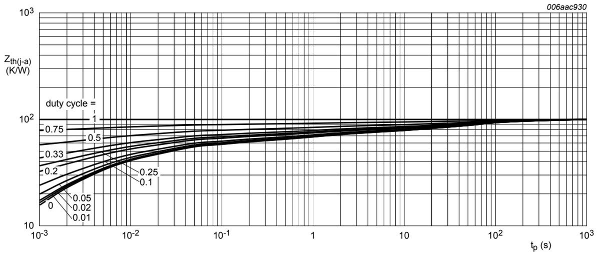
Ceramic PCB, Al<sub>2</sub>O<sub>3</sub>, standard footprint
