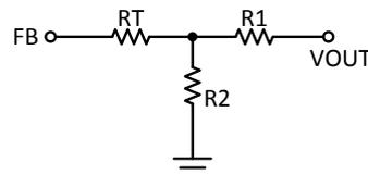
Figure 4: Structure of the feedback circuit.
