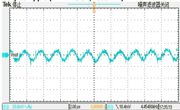
**Output Ripple (12V => 3.3V, Load=1A)**
