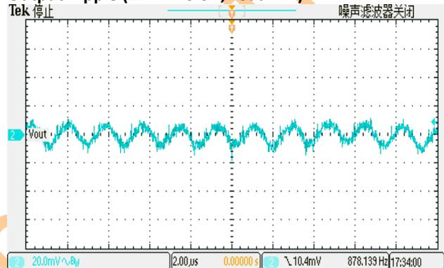
**Output Ripple (12V => 3.3V, Load=0A)**
