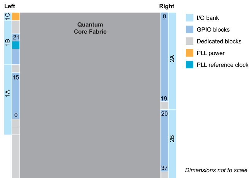
Figure 23: Floorplan Diagram for QFP144 Packages
