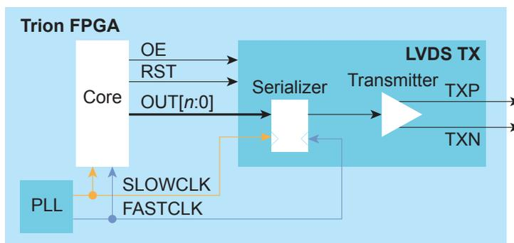
Table 16: LVDS TX Signals (Interface to FPGA Fabric)
