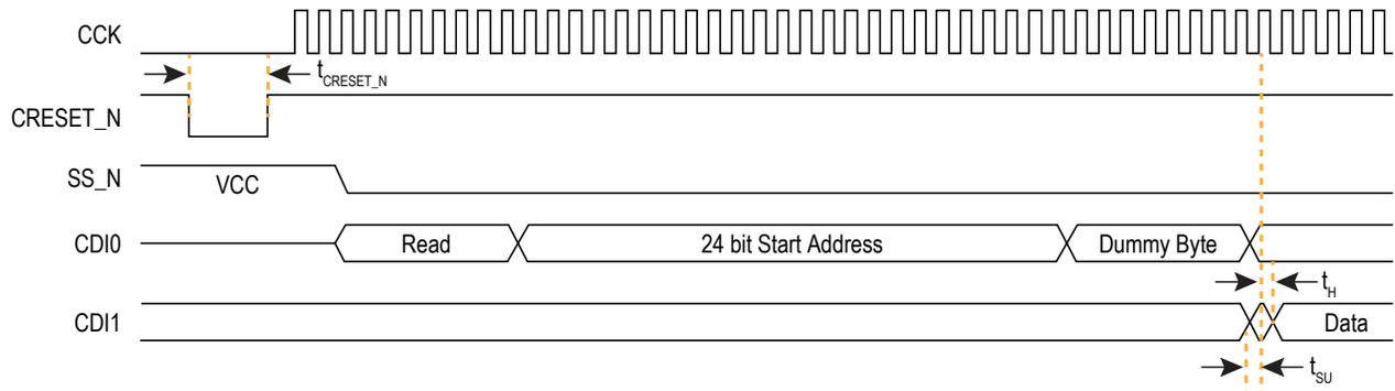
Figure 20: SPI Passive Mode (x1) Timing Sequence
