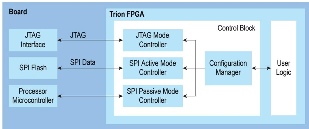
In active mode, the FPGA controls the configuration process. An oscillator circuit within the FPGA provides the configuration clock. The bitstream is typically stored in an external serial flash device, which provides the bitstream when the FPGA requests it.
