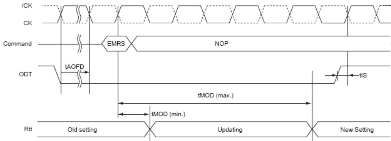
Note: tAOFD must be met before issuing EMRS command. ODT must remain low for the entire duration of tMOD window.
