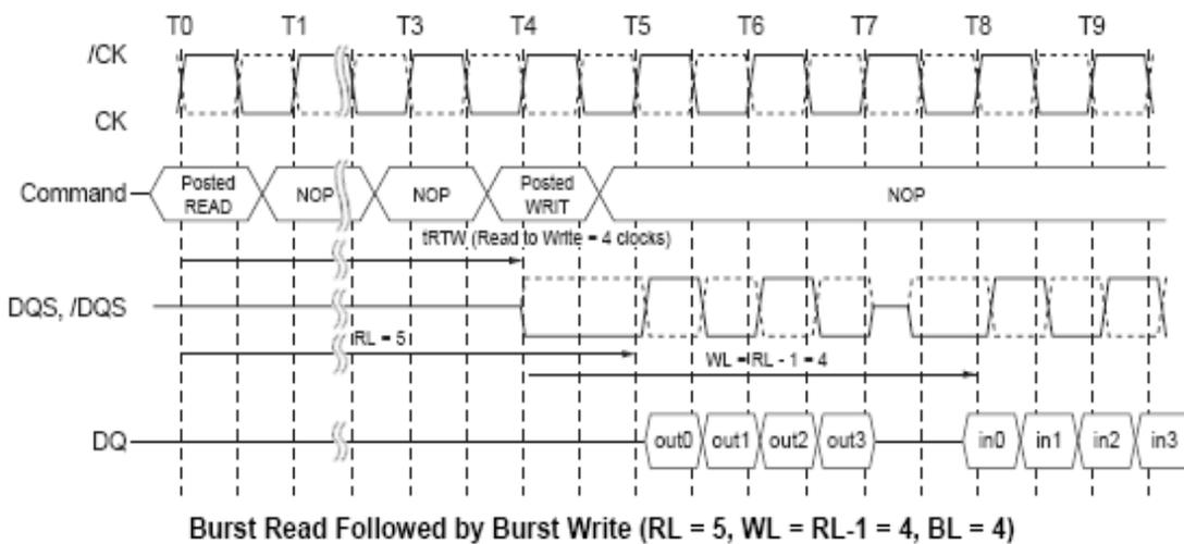
The minimum time from the burst read command to the burst write command is defined by a read-to-write-turn-around-time, which is 4 clocks in the case of BL = 4 operation, 6 clocks in case of BL =8 operation.
