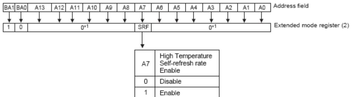
Note: 1 The rest bits in EMRS (2) is reserved for future use and all bits in EMRS (2) except A7, BA0 and BA1 must be programmed to 0 when setting the extended mode register (2) during initialization.
