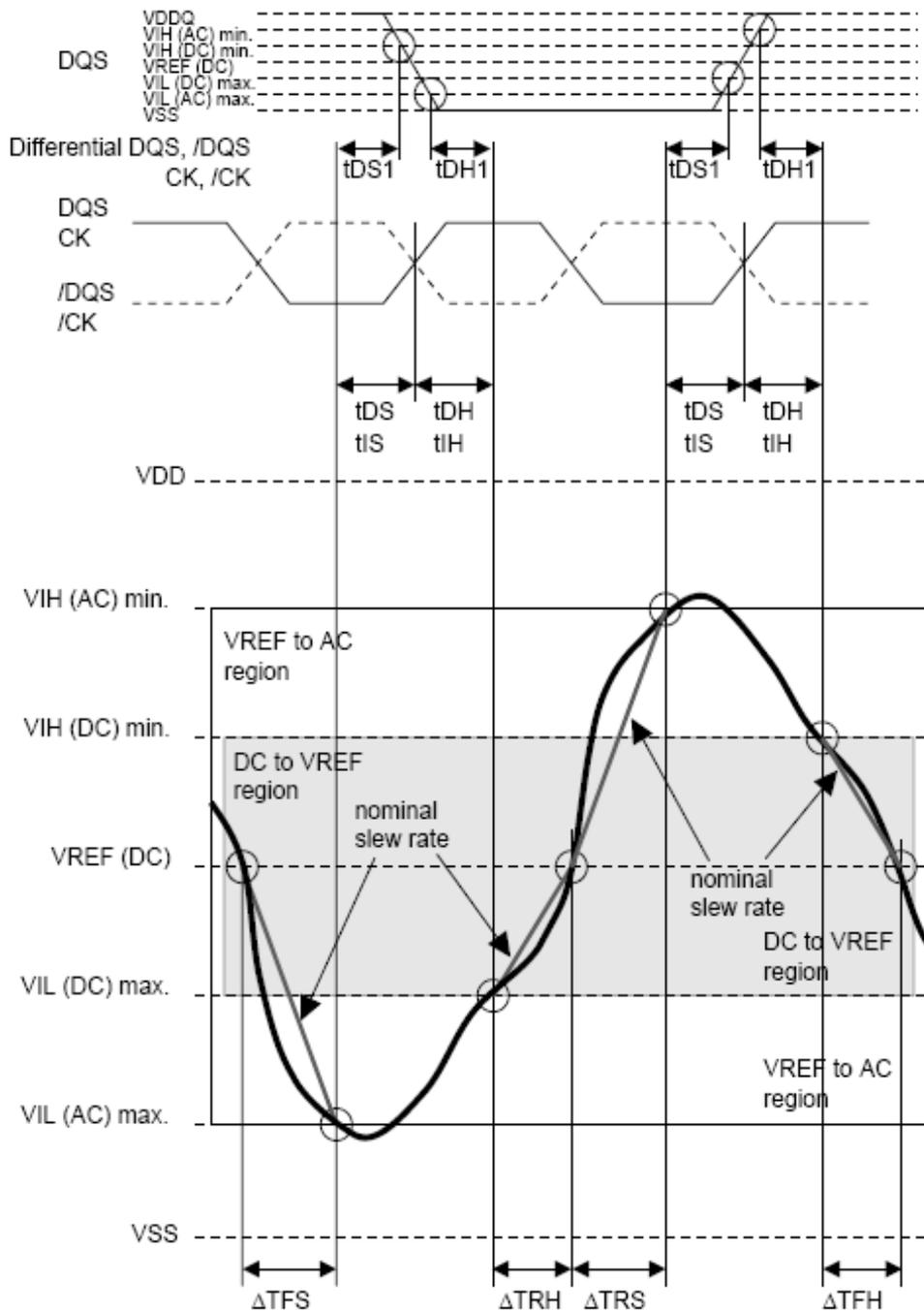
$$\text{Setup slew rate Falling signal} = \frac{VREF (DC) - VIL (AC) \text{ max.}}{\Delta TFS}$$
