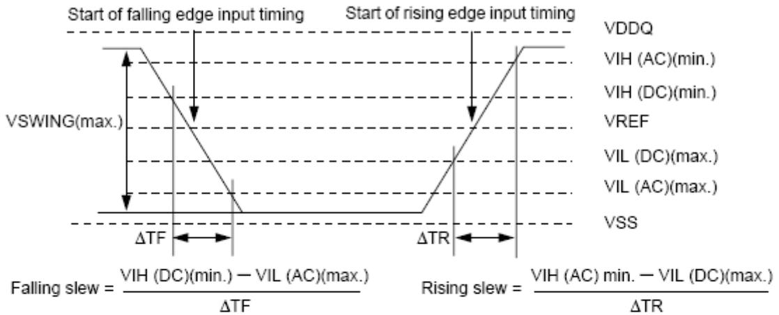
**AC Input Test Signal Wave forms**
