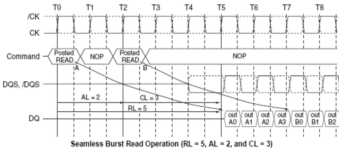
Enabling a read command at every other clock supports the seamless burst read operation. This operation is allowed regardless of same or different banks as long as the banks are activated.
