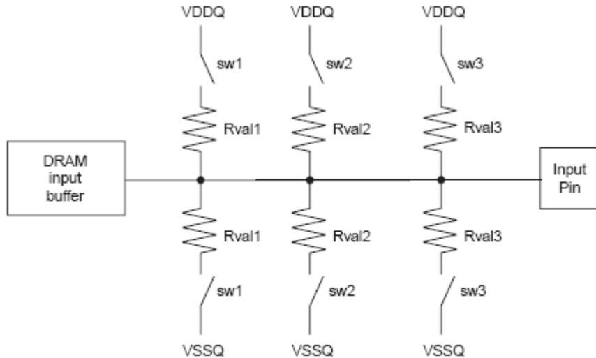
Switch sw1, sw2 or sw3 is enabled by ODT pin.
