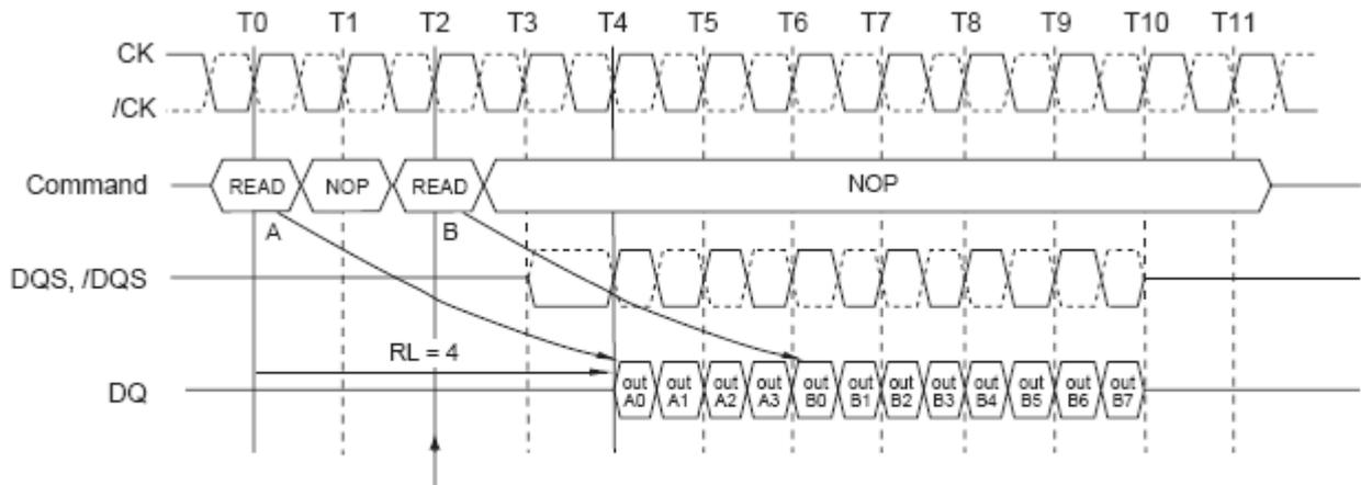
Burst interrupt is only allowed at this timing.
