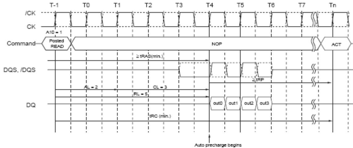
**Burst Read with Auto Precharge Followed by an Activation to the Same Bank (tRAS lockout case)**
