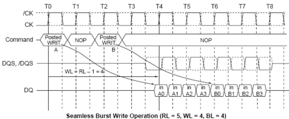
Enabling a write command every other clock supports the seamless burst write operation. This operation is allowed regardless of same or different banks as long as the banks are activated.
