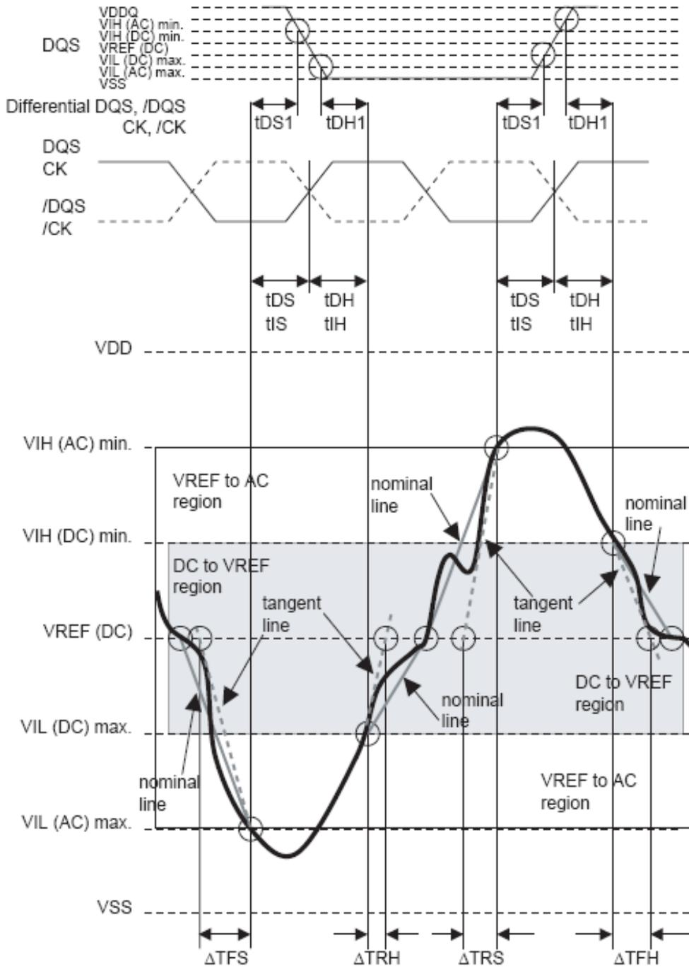
$$\text{Setup slew rate Falling signal} = \frac{\text{tangent line [VREF (DC) - VIL (AC) max.]} }{\Delta TFS}$$
