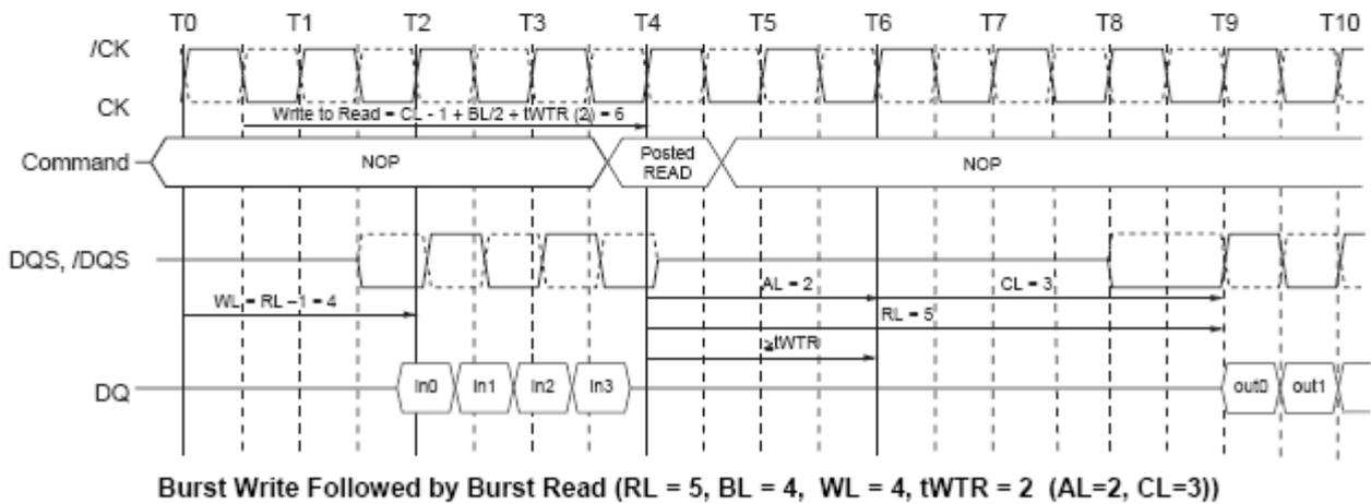
The minimum number of clock from the burst write command to the burst read command is  $CL - 1 + BL/2 +$  a write to-read- turn-around-time (tWTR). This tWTR is not a write recovery time (tWR) but the time required to transfer the 4bit write data from the input buffer into sense amplifiers in the array.
