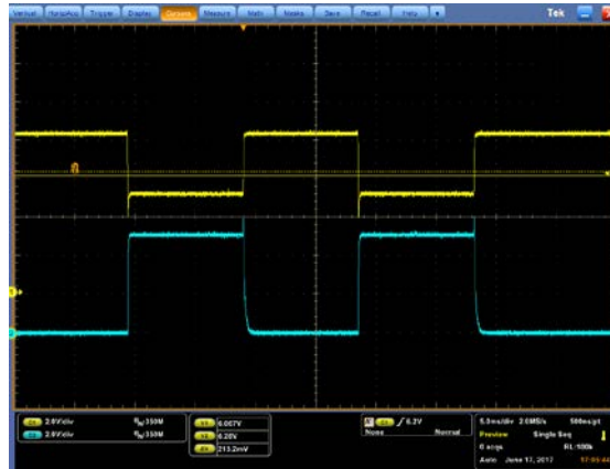
Fig3. OVP recovery waveform (OVP 6V)
