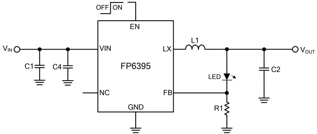
Figure 2. Schematic Diagram
