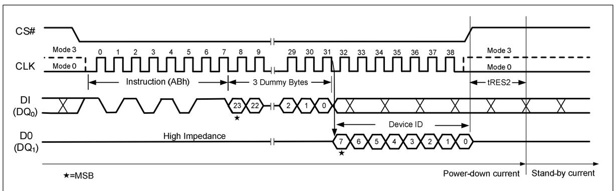
Figure 21 Release Power-down / Device ID Instruction
