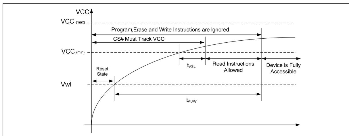
Figure 25 Power-up Timing
