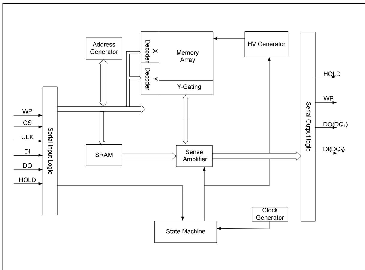
Figure 1 FM25F005 Serial Flash Memory Block Diagram
