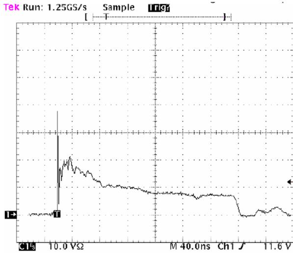
Figure 1. ESD Clamping Voltage Screenshot
