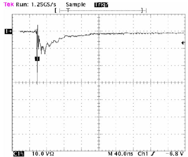
Figure 2. ESD Clamping Voltage Screenshot
