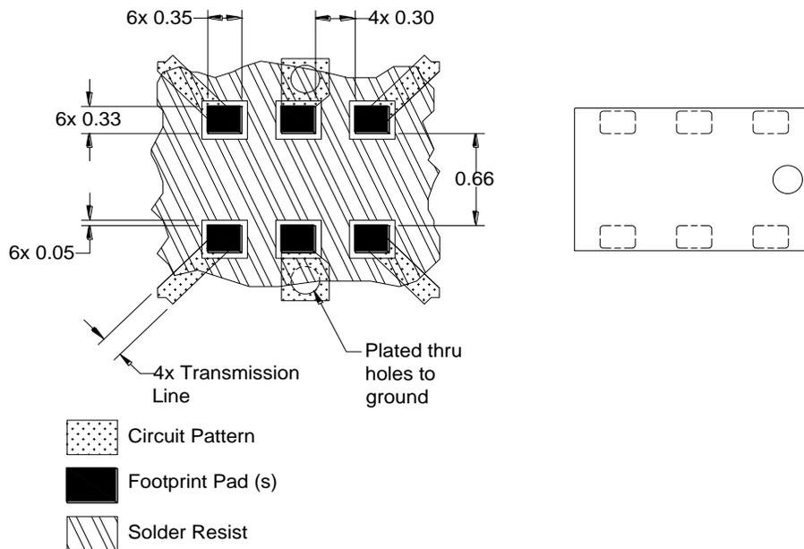
Dimensions are in Millimeters
