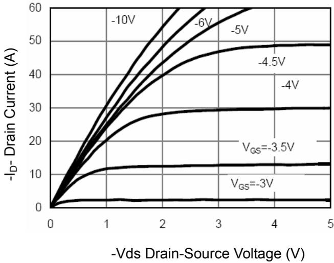
**Figure 1 Output Characteristics**
