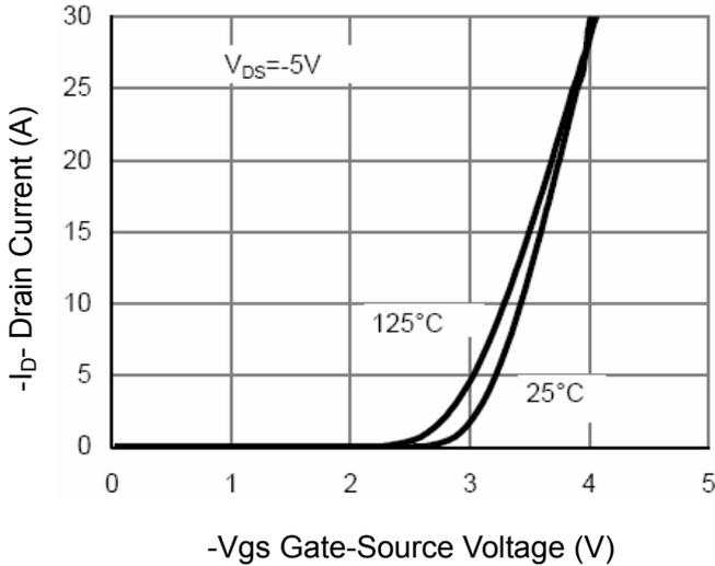
**Figure 2 Transfer Characteristics**
