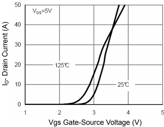
Figure 2 Transfer Characteristics
