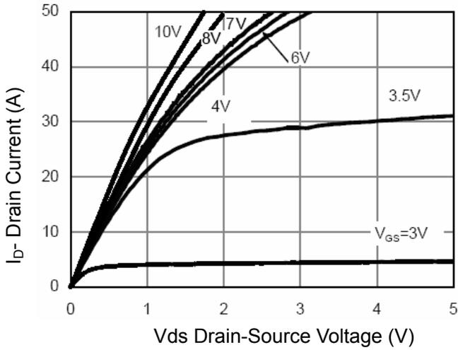
Figure 1 Output Characteristics
