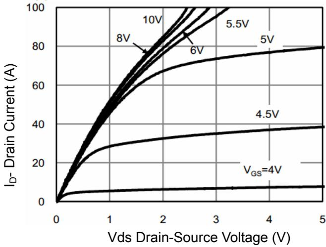
Figure 1 Output Characteristics
