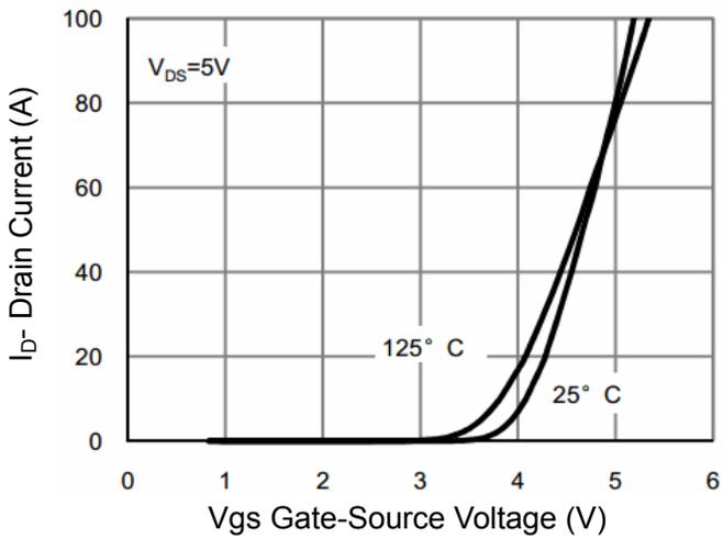
Figure 2 Transfer Characteristics
