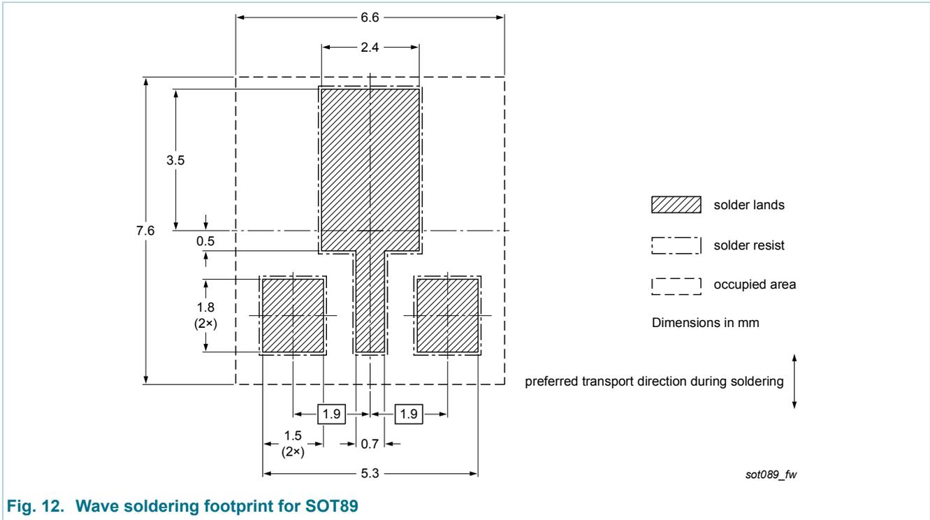
Fig. 12. Wave soldering footprint for SOT89
