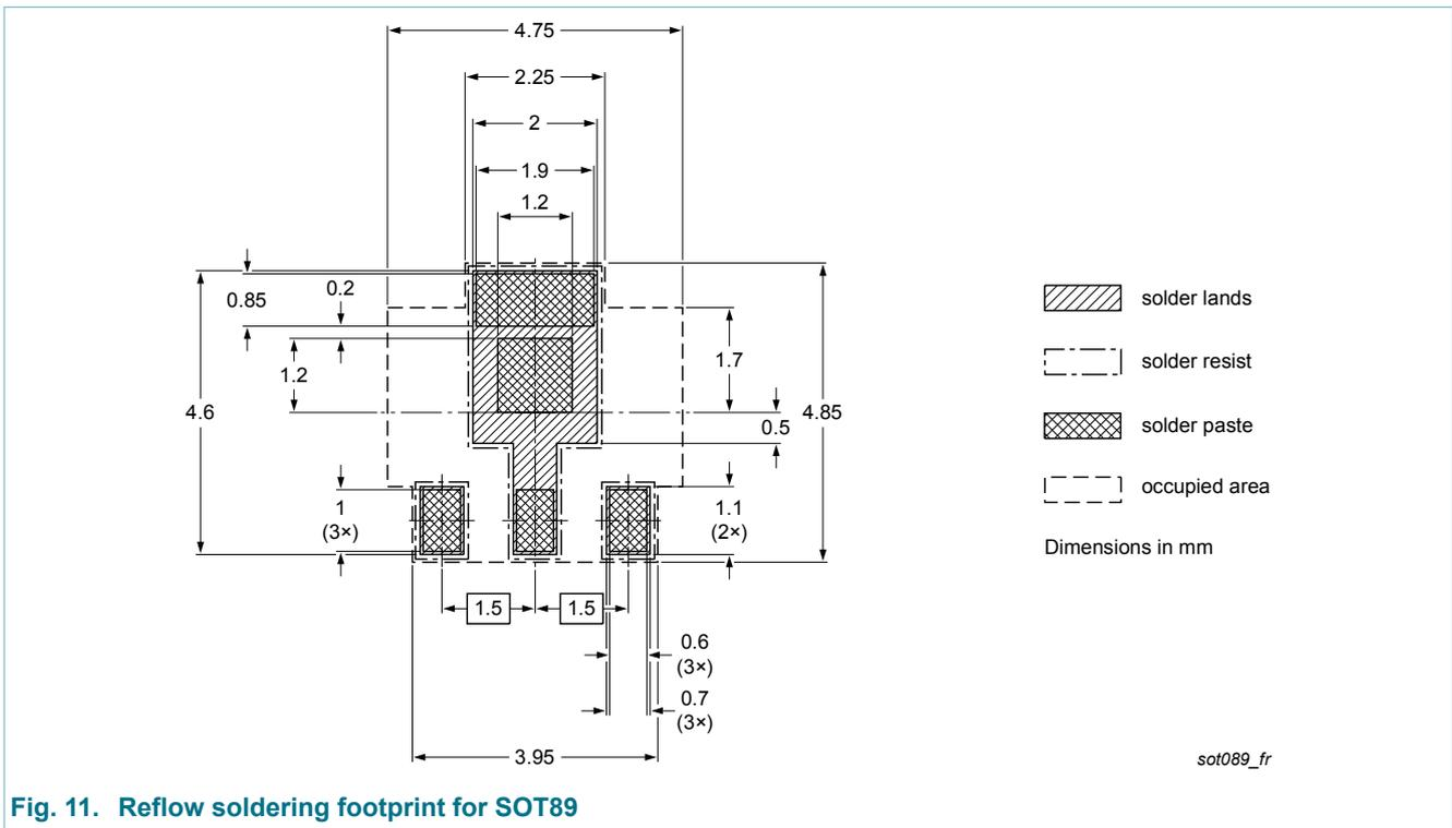
Fig. 11. Reflow soldering footprint for SOT89
