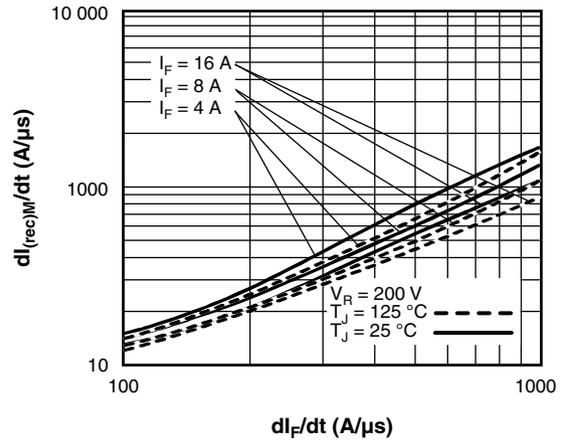
Fig. 8 - Typical  $di_{(rec)M}/dt$  vs.  $di_F/dt$  (Per Leg)
