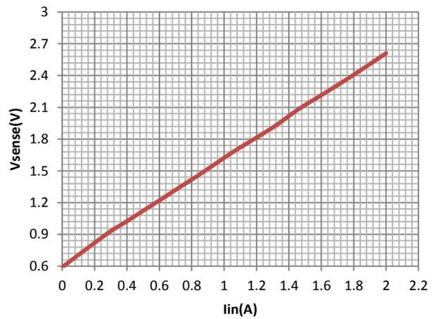
Figure 7. Current Sense Output Voltage vs Iin
