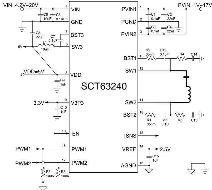
Figure 11. Separate Input to VIN and PVIN
