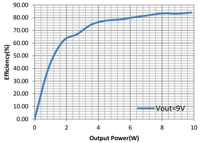
Figure 3. Transfer Efficiency with 10W RX@ Vout=9V
