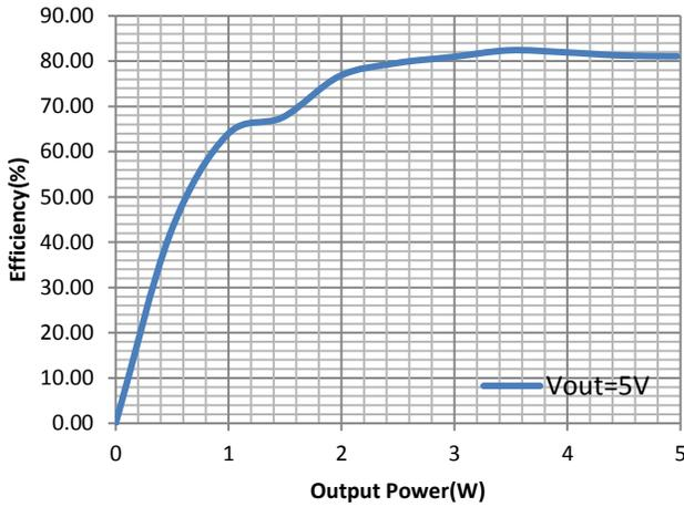
Figure 2. Transfer Efficiency with 5W RX@ Vout=5V
