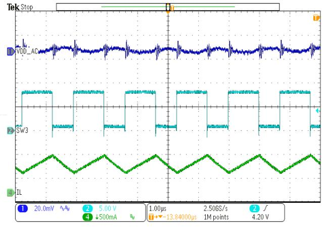
Figure 15. VDD Ripple and SW3 @VIN=9V, IOUT=600mA
