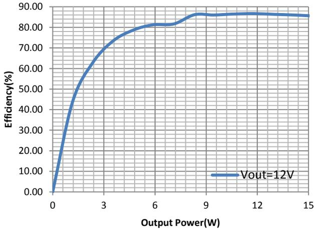
Figure 4. Transfer Efficiency with 15W RX@ Vout=12V
