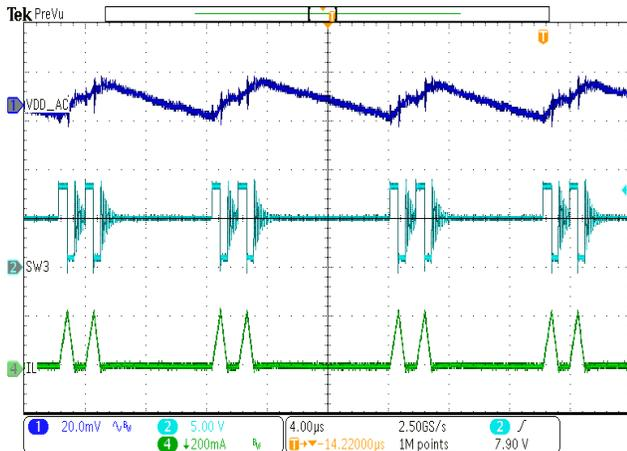
Figure 14. VDD Ripple and SW3 @VIN=9V, IOUT=20mA
