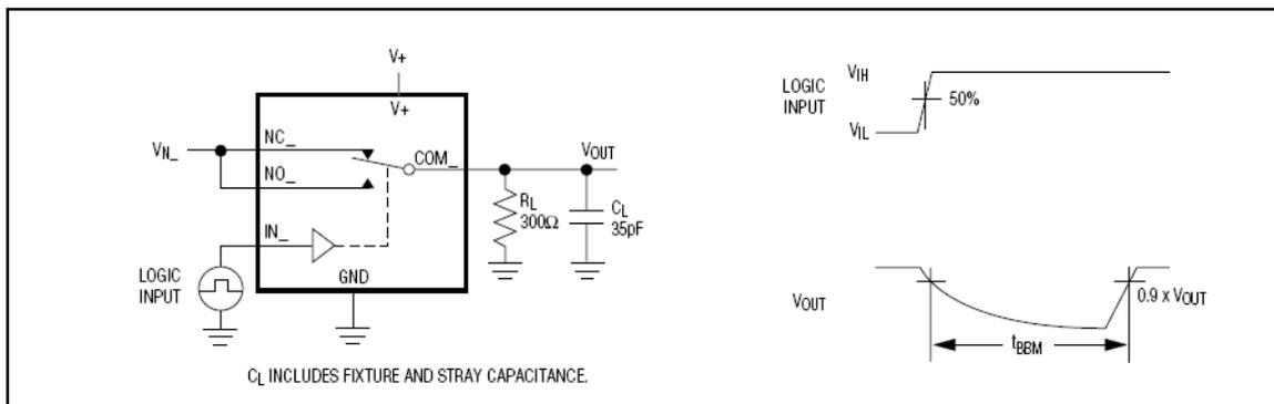
Figure 2. Break-Before-Make Interval
