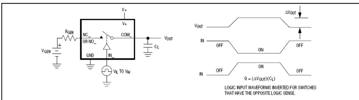
Figure 4. Charge Injection
