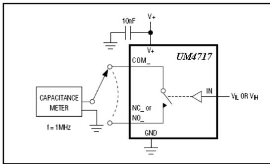
Figure 6. Channel Off/On-Capacitance
