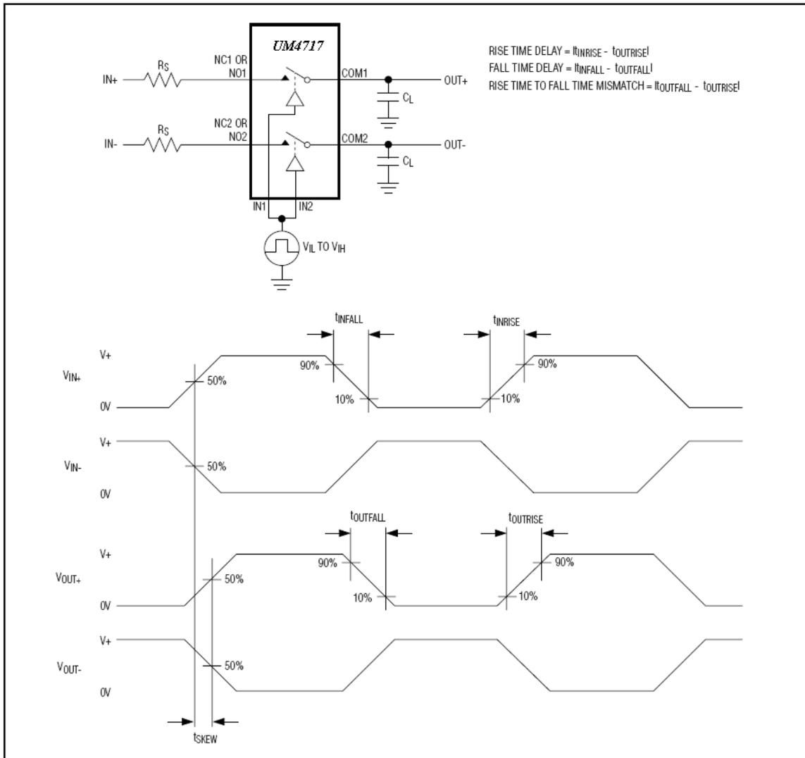
Figure 3. Output Signal Skew
